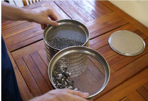
Figure 35 Sieve tower with 9 different mesh sizes
