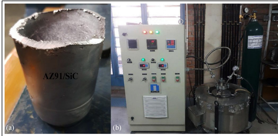
Figure 1. AZ91/SiC composites fabrication through stir casting: (a) AZ91/SiC composites and (b) stir casting set-up.
