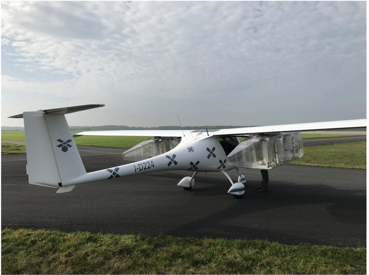
Fig 22. The aircraft used for detection, with the cargo boxes under the wings.
