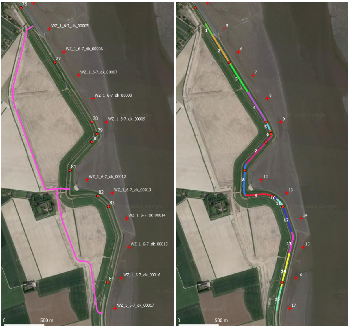
(a) Location of dike profiles (red dots) and Hydra-NL output locations (red crosses) (b) Sections and their corresponding ID. See Table 4.1 for the corresponding profiles and output locations.
