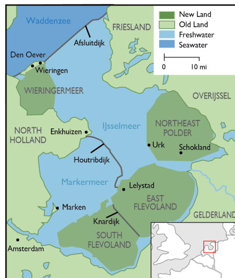
Figure 2.1: The Zuiderzee Works: The Afsluitdijk and multiple polders (Almere Tours, n.d.)
