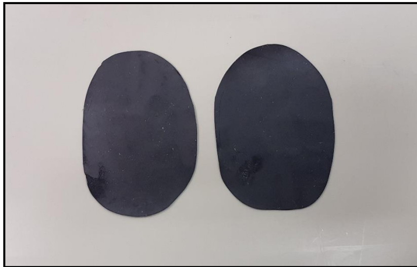
Fig. 5.3: Oval shaped hand-cut semi-conductive tapes
