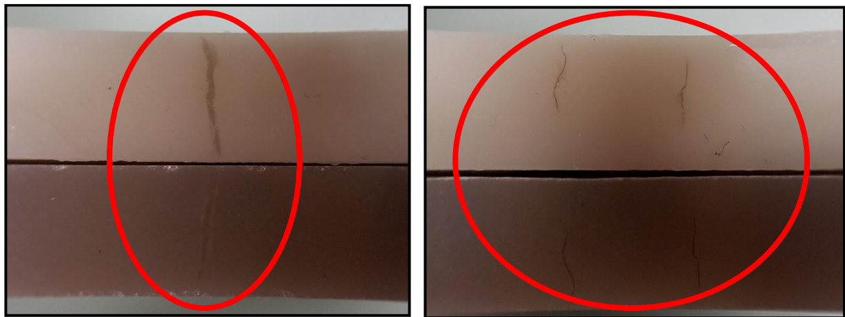
Fig. 5.21: AC breakdown path of heated samples - 0.5 bar [lower material- epoxy; upper material- silicon rubber]
