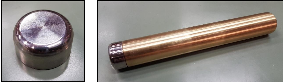
Fig. 4.19: Stainless steel electrode (left) and the entire electrode assembly (right)
