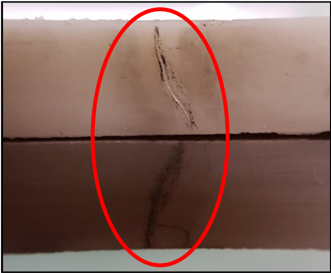
Fig. 5.7: AC breakdown path – 1 bar [lower material- epoxy; upper material- silicon rubber]
