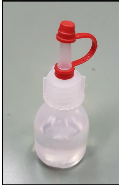
Fig. 5.11: Silicon oil used as a lubricant during installation
