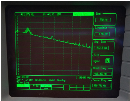
(a) Roll-off curve zoomed in at stop band. Marker at point A
