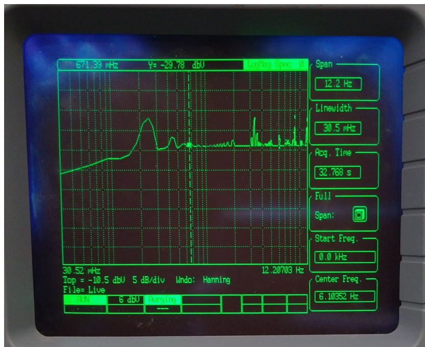
Figure 6.4: Filter response of the 6th-order Sallen-Key high-pass filter measured using a network analyzer and as a source: 10mV chirp
