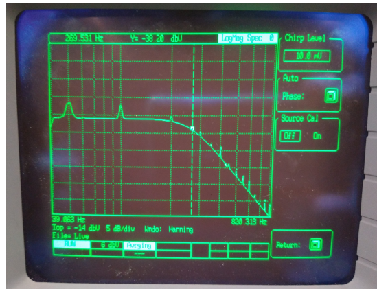
(b) Roll-off curve of the low-pass filter. Marker at -3dB point
