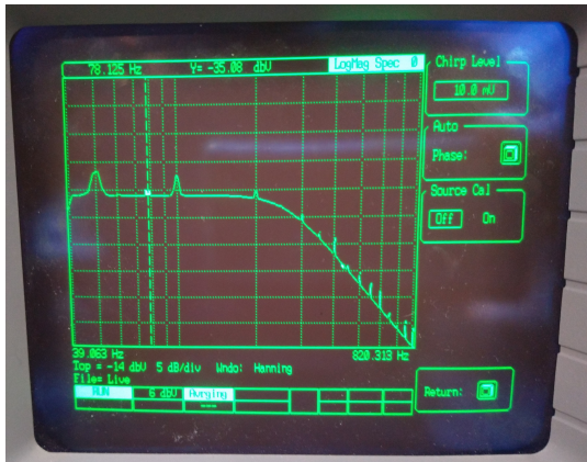
(a) Roll-off curve of the low-pass filter. Marker at pass-band
