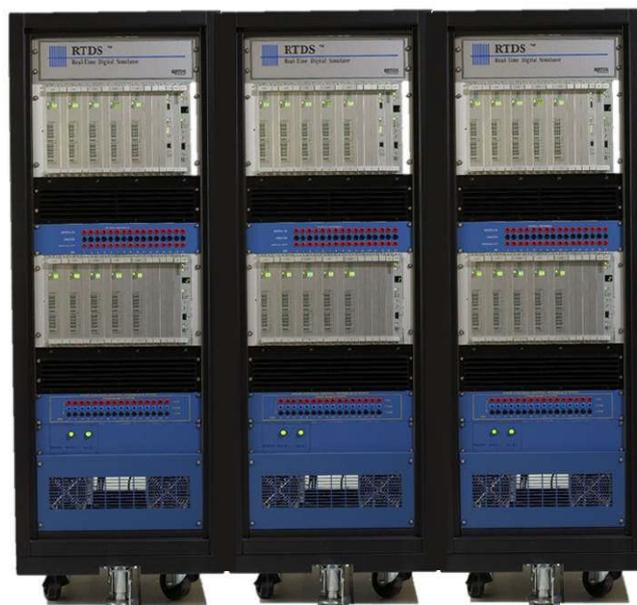
Figure B.1: A typical RTDS hardware setup
