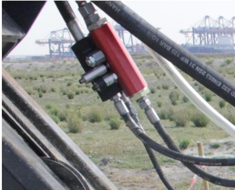
Figure 60: Hydraulic flow and pressure sensors
