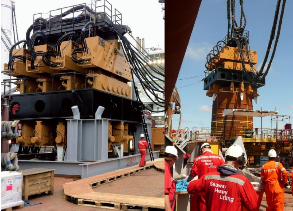
Figure 3: Vibratory hammer used for the Riffgat offshore windfarm project [11].
