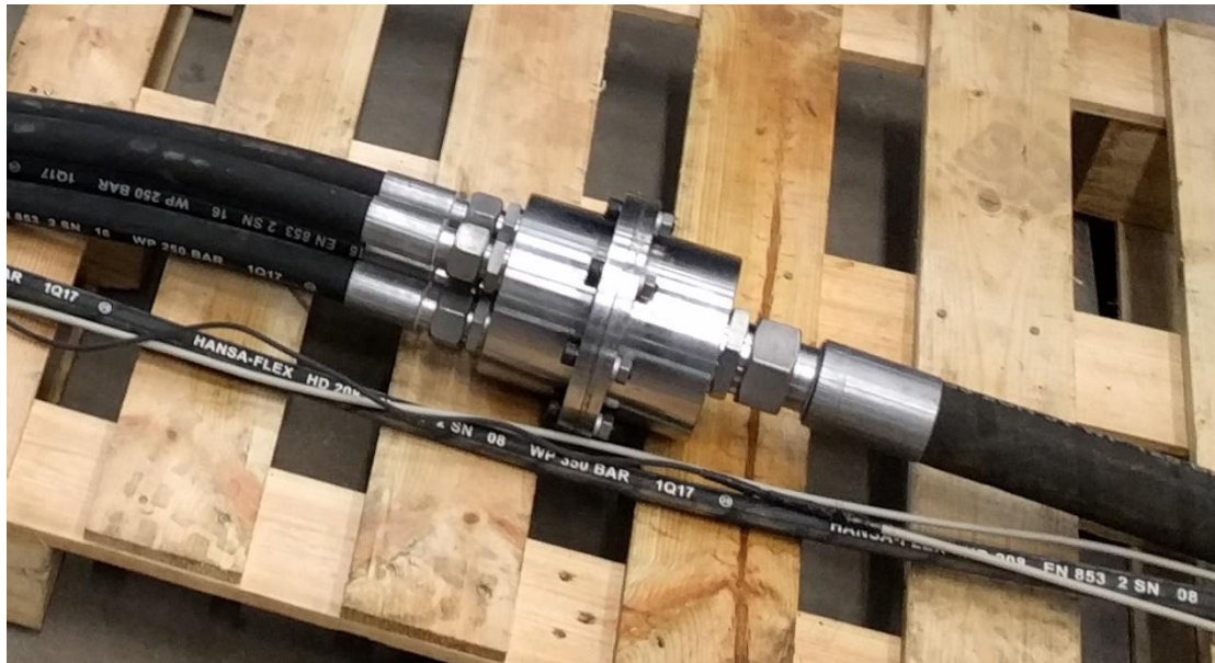
Figure 54: Water injection splitter
