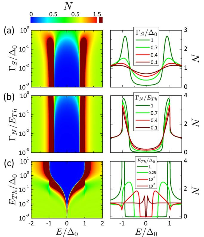
FIG. 3. DOS in the center of the three-terminal junction ( $x = 0$ ) calculated at zero fluxes,  $\Phi_L = \Phi_R = 0$ . (a) Dependence of the DOS on  $\Gamma_S/\Delta_0$  (fixed  $E_{Th}/\Delta_0 = 0.5$  and  $\Gamma_N/E_{Th} = 10^{-3}$ ). (b) Dependence of the DOS on  $\Gamma_N/E_{Th}$  (fixed  $E_{Th}/\Delta_0 = 0.5$  and  $\Gamma_S/\Delta_0 = 10^{-3}$ ). (c) Dependence of the DOS on the Thouless energy  $E_{Th}/\Delta_0$  (fixed  $\Gamma_S = \Gamma_N = 10^{-3}\Delta_0$ ).
