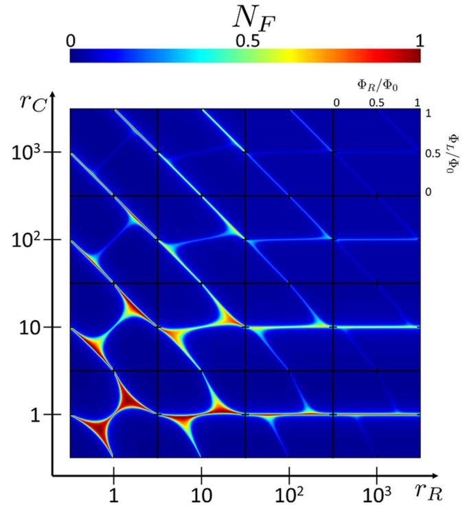
FIG. 6. Evolution of the DOS at the Fermi energy  $N_F(\Phi_L, \Phi_R)$  for different values of  $S/N$  interface opacities  $r_R$  and  $r_C$  reported in the  $x$  and  $y$  axis, respectively. Here  $r_L = 1$ ,  $E_{\text{Th}}/\Delta_0 = 0.5$ , and  $\Gamma_S = \Gamma_N = 10^{-3}\Delta_0$ .
