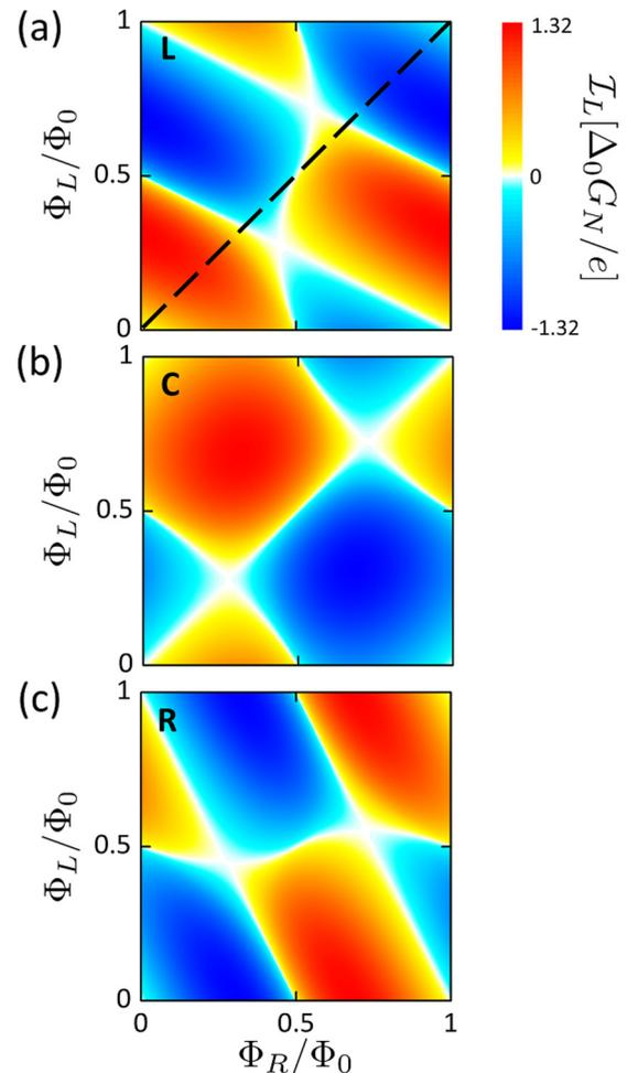
FIG. 9. Color plot of the supercurrents in each arm for different magnetic fluxes  $\Phi_R$  and  $\Phi_L$ . Here we have fixed  $E_{\text{Th}}/\Delta_0 = 5$  and  $\gamma_S = \gamma_N = 10^{-3}\Delta_0$ , and  $T = 0.02T_c$ . The supercurrents flowing out of the left, central, and right arm are plotted in (a), (b), and (c), respectively.
