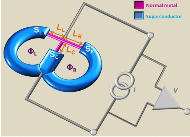
FIG. 1. Scheme of the  $\omega$ -SQUIPT in a current-biased setup.  $I$  is the current flowing through the circuit, and  $V$  is the voltage drop across the device.  $\Phi_L$  and  $\Phi_R$  represent the magnetic fluxes piercing the left and right loop, respectively.  $L_L$ ,  $L_C$ , and  $L_R$  refer to the left, center, and right arms length of the T-shaped normal metal, respectively. Finally,  $S_L$ ,  $S_C$ , and  $S_R$  refer to the left, center, and right superconducting leads.
