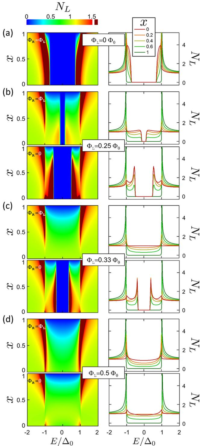
FIG. 5. Spatial dependence of the DOS evaluated at different fluxes, with  $E_{\text{Th}}/\Delta_0 = 0.5$  and  $\Gamma_S = \Gamma_N = 10^{-3}\Delta_0$ . Each central box indicates the value of the flux  $\Phi_L$  associated with the near plots; the top plots show the case of equal fluxes  $\Phi_R = \Phi_L$  and the bottom plots show the single flux case with  $\Phi_R = 0$ . (a)  $\Phi_L = 0$ ; (b)  $\Phi_L = 0.25\Phi_0$ ; (c)  $\Phi_L = 0.33\Phi_0$ ; and (d)  $\Phi_L = 0.5\Phi_0$ .
