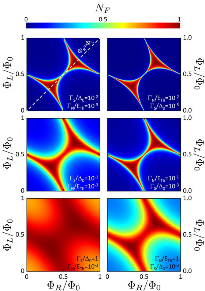
FIG. 2. Evolution of the DOS at the Fermi energy  $N_F(\Phi_L, \Phi_R)$  for increasing pair-breaking scattering both in the  $S$  leads,  $\Gamma_S$  (left column), and in the  $N$  weak link,  $\Gamma_N$  (right column). The values of  $\Gamma_N/E_{Th}$  and  $\Gamma_S/\Delta_0$  are reported in each panel. The weak link is of an intermediate length  $E_{Th}/\Delta_0 = 0.5$  and the  $S/N$  interfaces are transparent.
