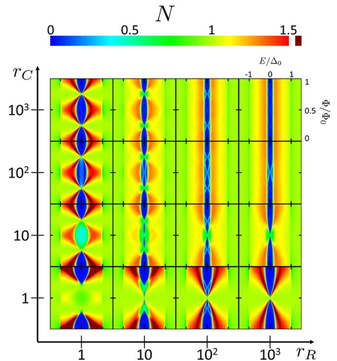
FIG. 7. Energy spectrum of the DOS as a function of equal fluxes  $\Phi_L = \Phi_R \equiv \Phi$  and calculated for different values of  $S/N$  interface opacity  $r_R$  and  $r_C$  reported in the  $x$  and  $y$  axis, respectively. Here  $r_L = 1$ ,  $E_{\text{Th}}/\Delta_0 = 0.5$ , and  $\Gamma_N = \Gamma_S = 10^{-3}\Delta_0$ .
