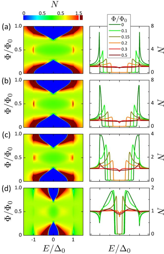
FIG. 4. DOS calculated in the middle of the three-terminal junction ( $x = 0$ ) for equal fluxes  $\Phi_L = \Phi_R \equiv \Phi$  with  $\Gamma_S = \Gamma_N = 10^{-3}\Delta_0$ . Each panel corresponds to a different Thouless energy: (a)  $E_{\text{Th}}/\Delta_0 = 5$ ; (b)  $E_{\text{Th}}/\Delta_0 = 1$ ; (c)  $E_{\text{Th}}/\Delta_0 = 0.5$ ; and (d)  $E_{\text{Th}}/\Delta_0 = 0.1$ .
