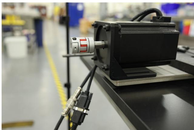
**Fig. 3** Inner shaft connected to the stepper motor
