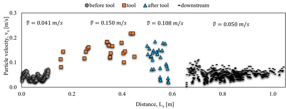
**Fig. 14** Average particle velocity ( $\bar{v}$ ) from image processing; for the case of 9.8 L/min and 120 RPM
