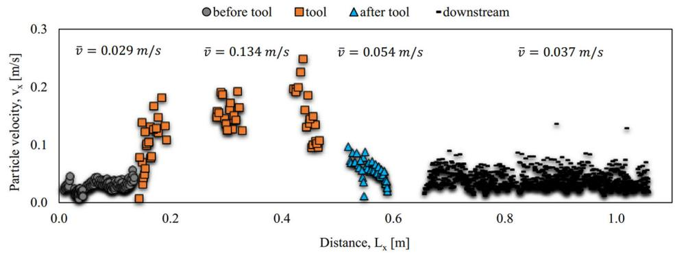
**Fig. 12** Average particle velocity ( $\bar{v}$ ) from image processing; for the case of 9.8 L/min and 80 RPM
