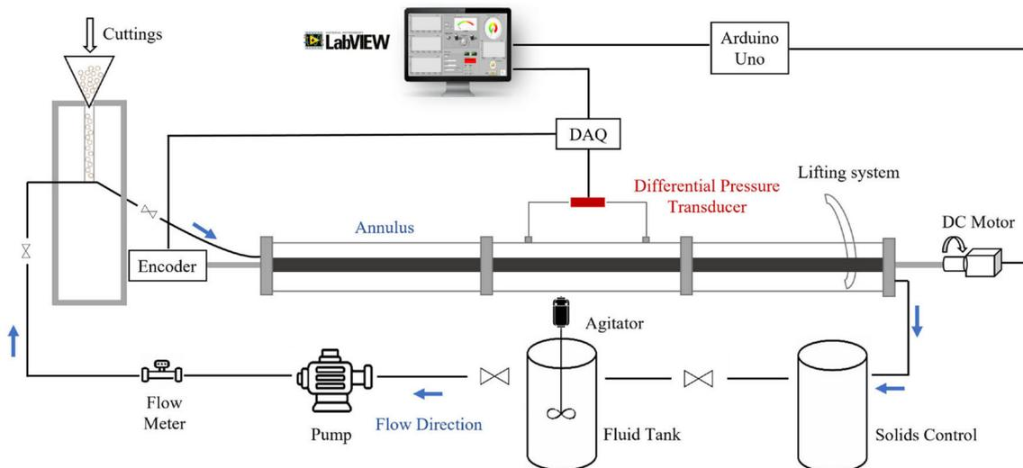
Fig. 6 Schematic diagram of custom-built flow loop setup
