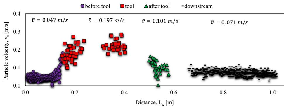
**Fig. 16** Average particle velocity ( $\bar{v}$ ) from image processing; for the case of 13.2 L/min and 80 RPM
