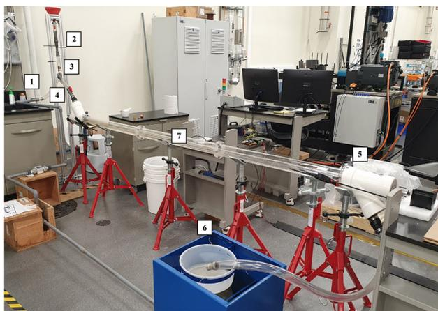
**Fig. 8** Actual flow loop design. The main control valves, as depicted, are: (1) entrance valve–fluid, (2) entrance valve–cuttings, (3) entrance control valve–fluid + cuttings, (4) additional safety control valve, (5) relief valve, and (6) end valve. The clamp-on tool is positioned within the central test section and clamped onto the inner pipe (7)
