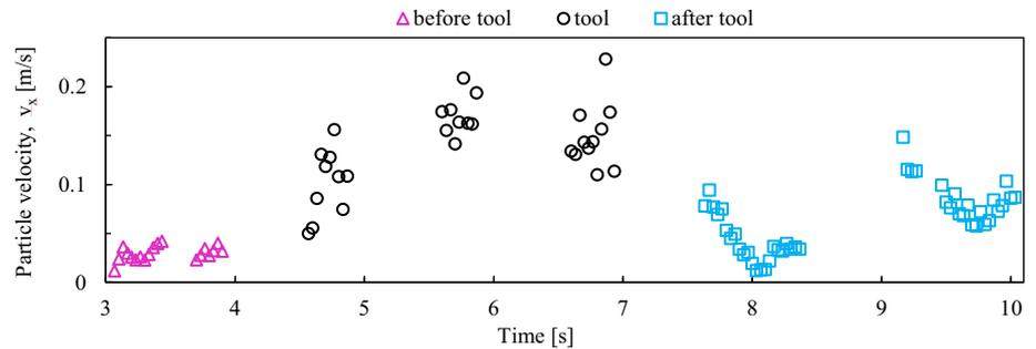
**Fig. 11** Average particle velocity ( $\bar{v}$ ) from image processing; for the case of 9.8 L/min and 60 RPM
