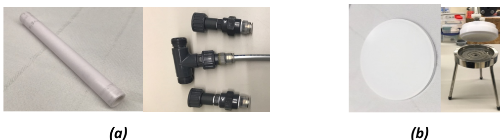
Fig 3.1 Pristine ceramic membranes with different configurations and corresponding membrane holders
