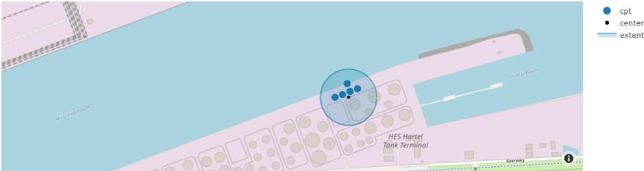
(b) Plan view of the CPTs that were selected at Section D of the HHTT quay wall
