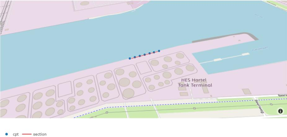
(b) Plan view of the CPTs that were selected at Section D of the HHTT quay wall
