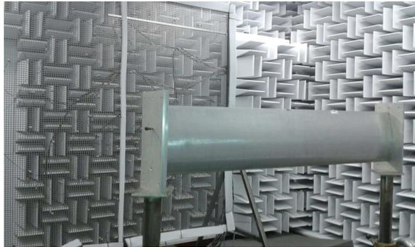
Figure 4.4: Wing used as obstacle in the noise shielding measurements.
