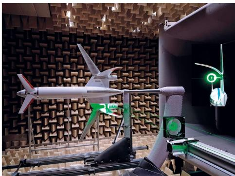
Figure 1.3: Top view of a scale model of DLR's Low Noise Aircraft in the Low-speed wind tunnel Braunschweig (NWB) operated by the foundation Deutsch-Niederländischer Windkanal (DNW) [29].
