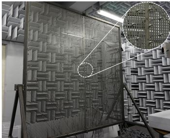
(a) Microphone array used in the experiments [45].
