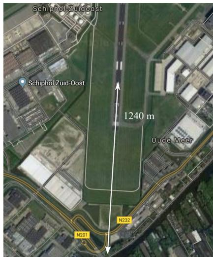
Figure 3.1: Microphone array location, at 1240 m to the South from the Aalsmeerbaan runway, at Amsterdam Airport Schiphol.
