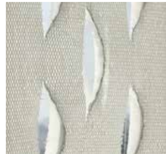
FIG. 12 Spacer textile, cover surfaces stretchable in opposite directions
