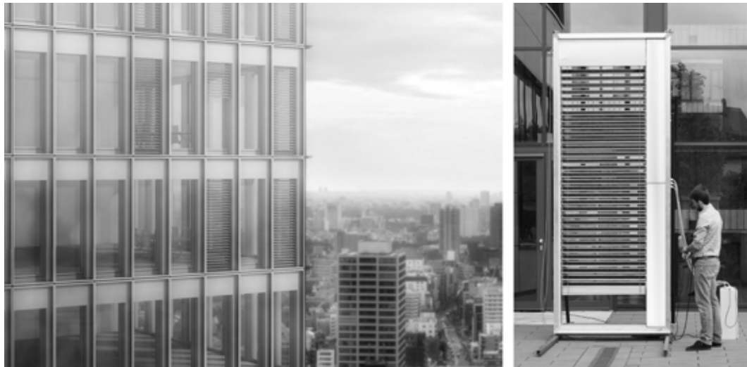
FIG. 11 Visual impression of DSF with integrated STVB (left) © IBK2. Current stage of LabTestSample (right) © Fraunhofer ISE
