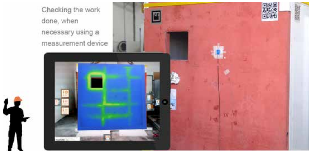
FIG. 2 INSITER mobile App for BIM-based Augmented Reality
