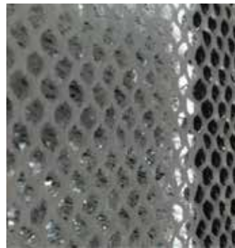
FIG. 14 Spacer textile with side-based magnetically activatable colour particles
