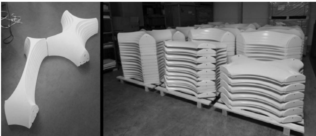
FIG. 5 Efficiently stacked basic light-weight elements after vacuum-formed molding in Germany, ready for transportation
