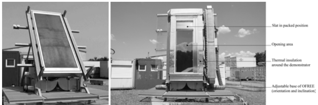
FIG. 3 OFREE without test sample. The black area is the measuring surface (left). The completed LabTestSample mounted on OFREE (right) © Fraunhofer ISE
