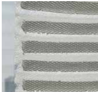
FIG. 10 Spacer textile, offset cut and stretched
