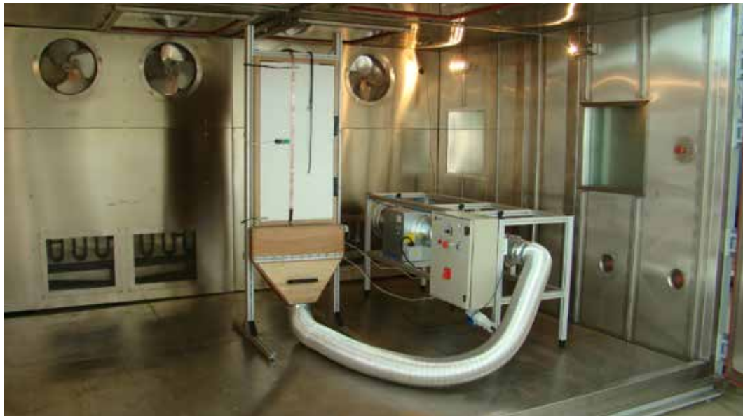
FIG. 3 First prototype of the ventilation unit and test area equipped with different sensors for experiments under defined climate conditions (placed in a climate chamber)
