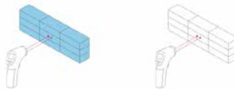
FIG. 5 Surface temperature was measure by infrared thermometer for both wet and dry bricks
