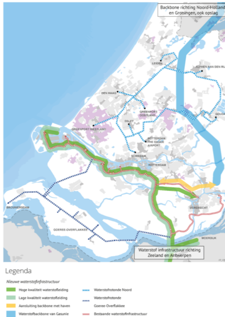
Figure 10.12: Map of proposed hydrogen transport infrastructure in South-Holland (van Wijk et al., 2019)
