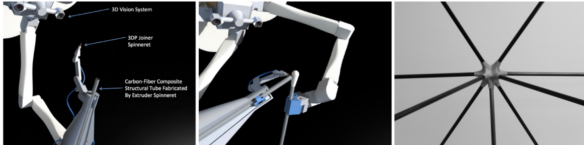
Figure 13.4: SpiderFab spinneret 3D-printing an optimized joint. Courtesy of Tethers Unlimited, Inc.
