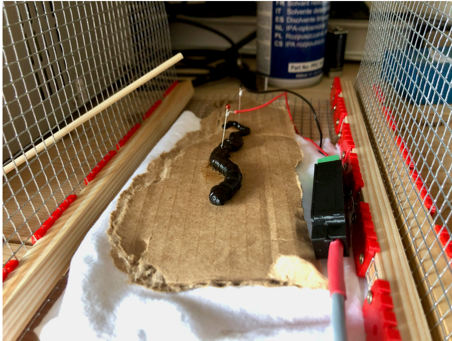
Figure 2.45: Setup overview to measure APs in a lugworm. The needles were placed inside the ventral nerve cord and connected to the preamplifier. The lugworm was placed inside the Faraday cage. A wooden chopstick to provoke APs is shown on the left.
