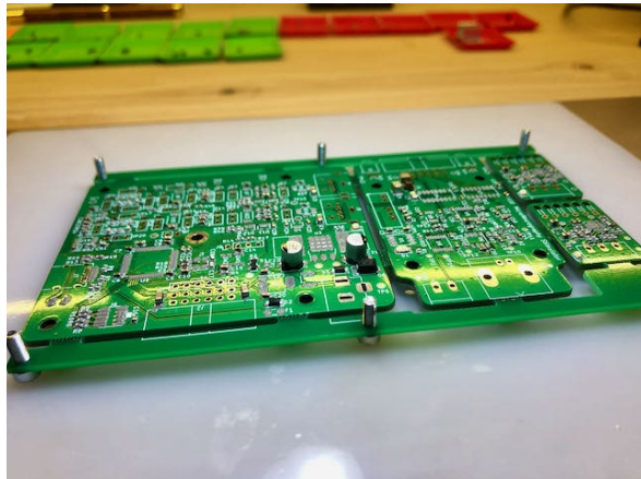
(d) The solder paste is applied, and some surface mount devices (SMD) are already placed.
