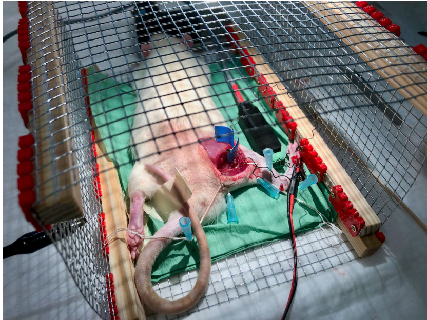
Figure 2.52: Setup overview for the second experiment. The rat was placed inside the Faraday cage. Two reference electrodes were used: one is placed in the sciatic nerve and one inside the surrounding tissue.
