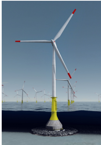
Figure 2.26: Seator tower Gravity based offshore wind turbine foundation with scour protection Source: Seator tower
