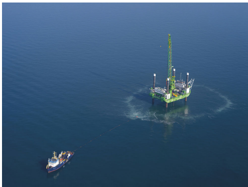
(a) GeoSea vessel Goliath working with big bubble curtain for Borkum West II
