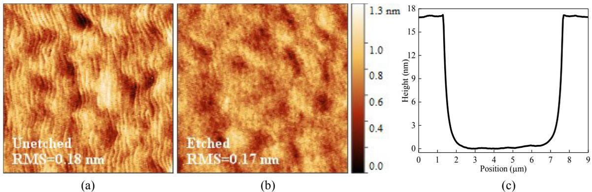
Fig. 3. AFM surface morphology images of (a) unetched and (b) etched surfaces using AST 450/150 (ICP/RF) recipe and (c) etched profile after 3 oxidation/etching cycles (c).
