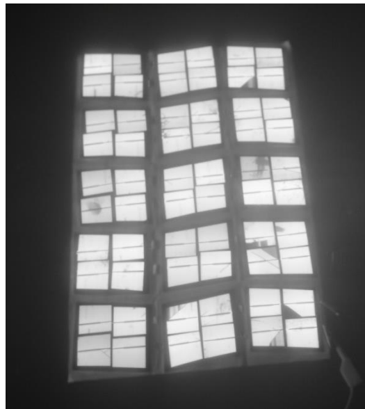
Figure 65. Electroluminescence analysis of the foldable module. It can be seen that the module suffered some damage during manufacturing (dark areas). Also, some cracks were formed during lamination and the cells themselves have some defects that appear as irregular spots.
