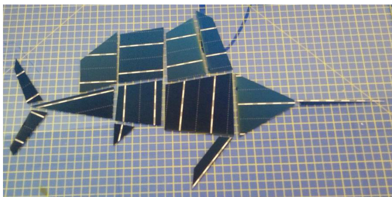
Figure 70. Cut cells prior to soldering and encapsulation.
