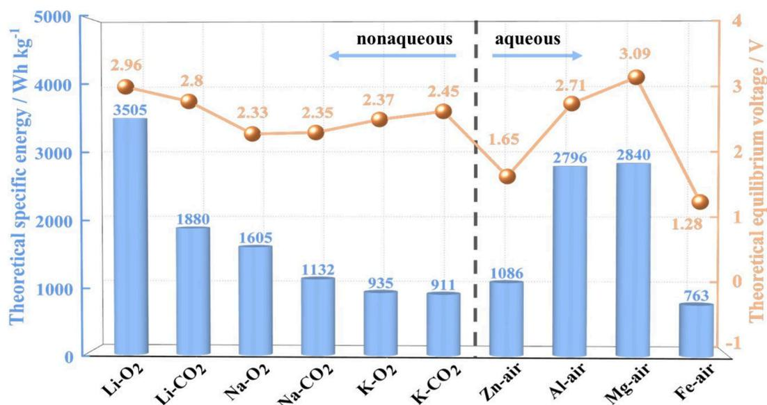
**Figure 1.** Theoretical specific energies and thermodynamic equilibrium potentials of nonaqueous electrolyte-based metal (Li, Na, K)-O<sub>2</sub>/CO<sub>2</sub> batteries and aqueous electrolyte-based metal (Zn, Mg, Al, and Fe)-air batteries. Specific energy densities are calculated based on total weight of the discharge products.
