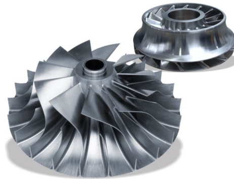
Figure 7.3: Unshrouded compressor impeller (front left) vs shrouded compressor impeller (right) [78]
