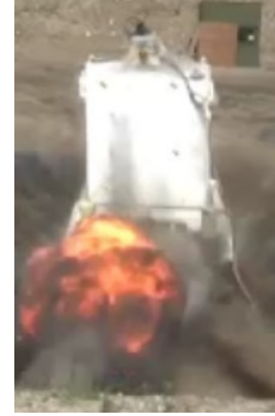
(b) The test rig during an experiment, one can see the soil ejecta and the ignition of detonation products. It can be seen that the test rig jumps upwards.
