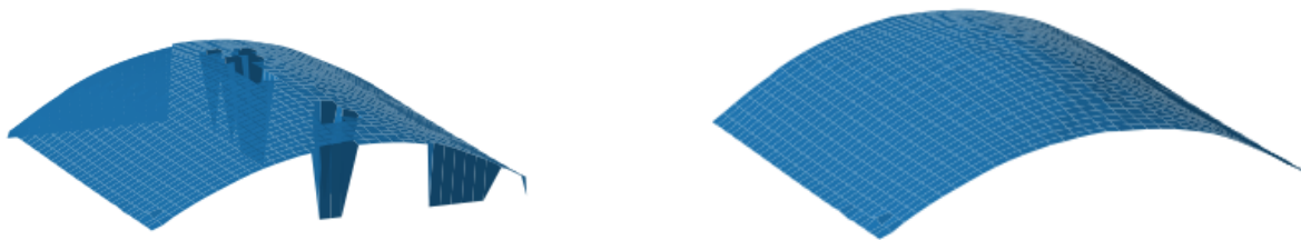
(a) DIC data directly interpolated from '.stl' mesh file to rectangular grid.
