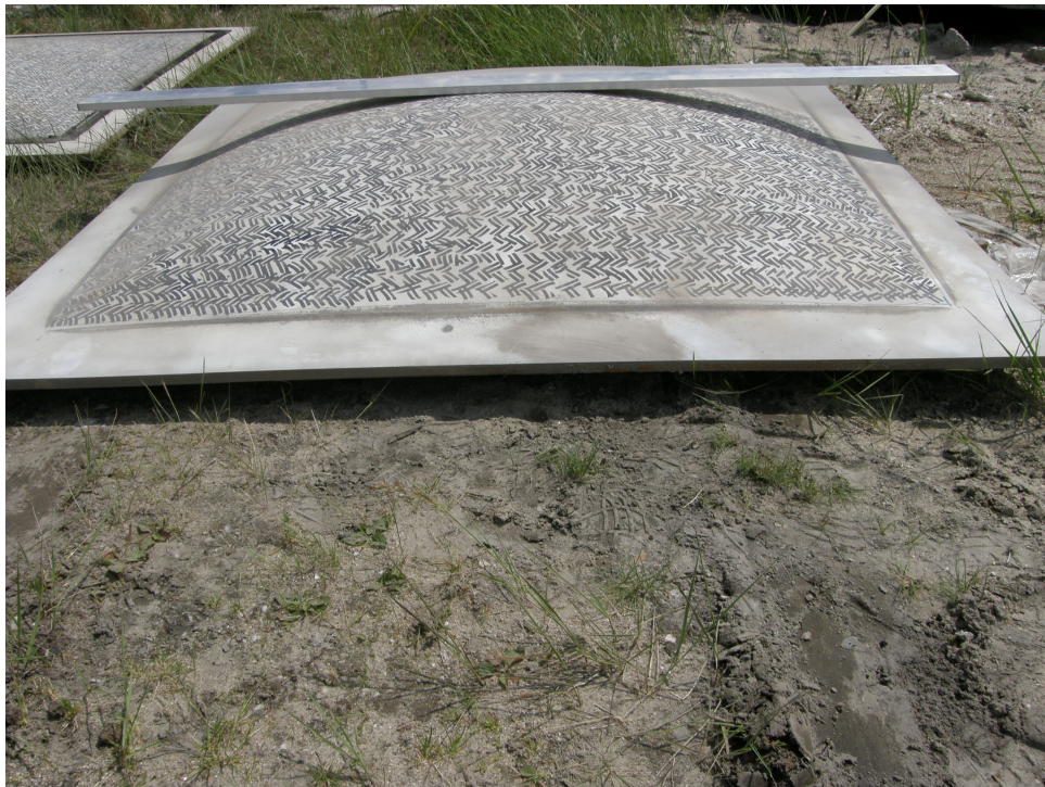
Figure 1.4: The image shows a plate after an experiment. The top of the plate is marked with a somewhat random pattern necessary for the DIC measurements. The straight bar positioned on top emphasizes that the plate has a large final deformation. Non linear modeling due to material non-linearity will be required.
