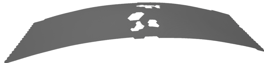
Figure 9.2: Output mesh of measured displacement from post processing the DIC data using ‘Gom-inspect’. The displacement is shown for t=T and hence the quality is less since the mesh shows four holes in the data.
