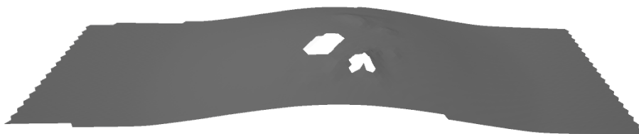
Figure 9.1: Output mesh of measured displacement from post processing the DIC data using ‘Gom-inspect’. The mesh shows two holes in the data that need to be interpolated. The displacement is shown for t=\frac{T}{2} .
