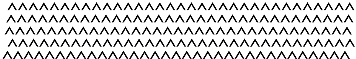
Figure 1.3: Example for an array of chevron-shaped protrusions, geometry based on Sirovich and Karlsson (1997)
