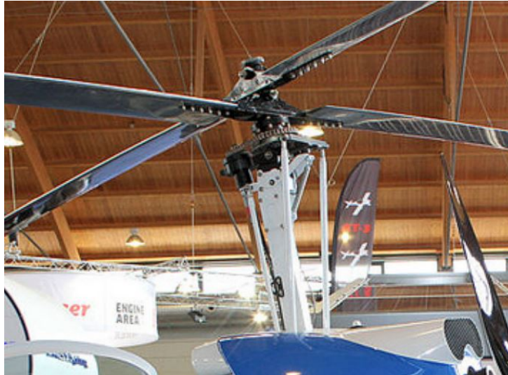
Figure 8.12: A close-up view of the Cloud Dancer II hub [53]
