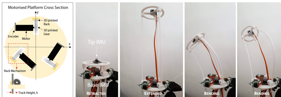
Fig. 2. Design of the actuation stages of the manipulator showing the triaxial motors and 3D printed tracks. Accompanied by pictures showing the range of motions and actions that can be achieved using the manipulator. The placement of the IMUs is highlighted.
