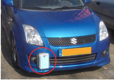
Fig. 2: Experimental auto equipped with NXP radar demonstrator
