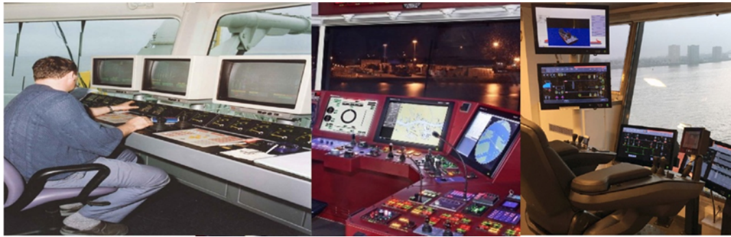
Figure 3: The evolution of HMI of dredge operator cockpit: (1) Dredge operator cockpit in 1990s (2) Dredge operator cockpit in 2000s (3) Dredge operator cockpit nowadays
