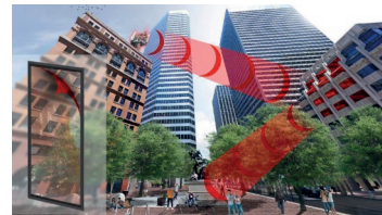
Figure 6.2: Transparent screen antenna reflects signal to cover dead zones [220].
