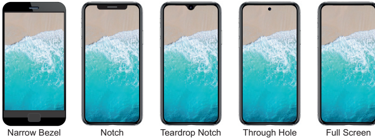
Figure 1.1: Illustration of the screen evolution of smartphones: efforts made to eliminate the notch and bezel.
