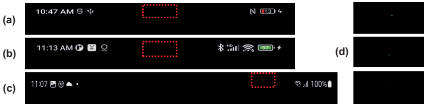
Figure 4.10: Screenshots of the smartphone status bar when running the one-pixel perturbation on (a) ZTE AXON30, (b) Xiaomi MIX4, and (c) Samsung Fold4. The transparent screen region is highlighted by the red dotted rectangle, and magnified in (d). These changes are imperceptible.
