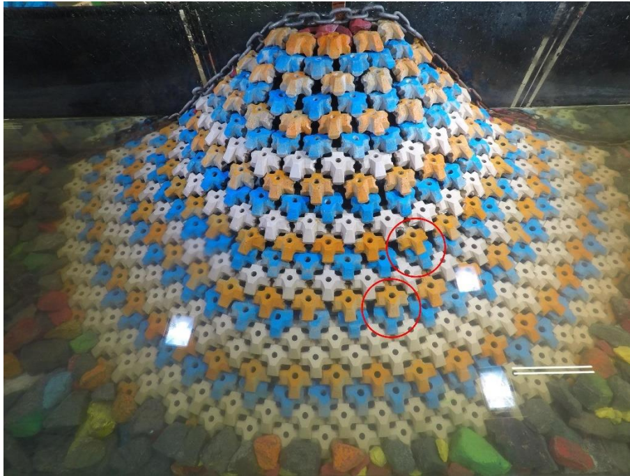
Figure 6.3. Unfavourable positioning of column-positioned XP-Base and XP-Curve due to settlements and a large D_x . The lower marked pair initiated failure.
