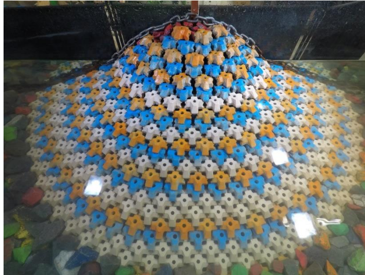
Figure D.26. Structure after 0.8 H_{m0} test run of Series 1.3 ( N_s = 1.82 ).
