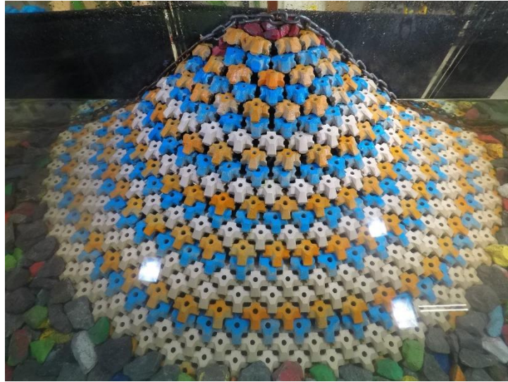
Figure D.23. Structure after 1.1 H_{m0} test run of Series 1.2.2 ( N_s = 2.72 ).
