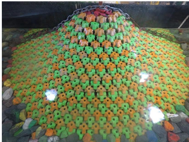
Figure D.65. Structure after 0.8 H_{m0} test run of Series 2.4 ( N_s = 2.04 ).
