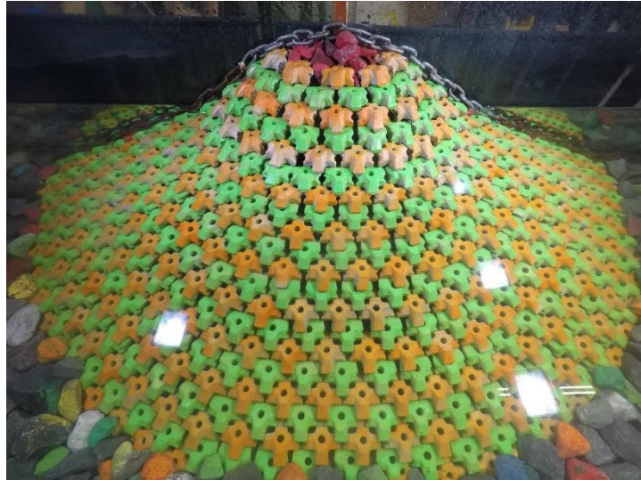
Figure D.58. Structure after 0.8 H_{m0} test run of Series 2.3 ( N_s = 1.92 ).
