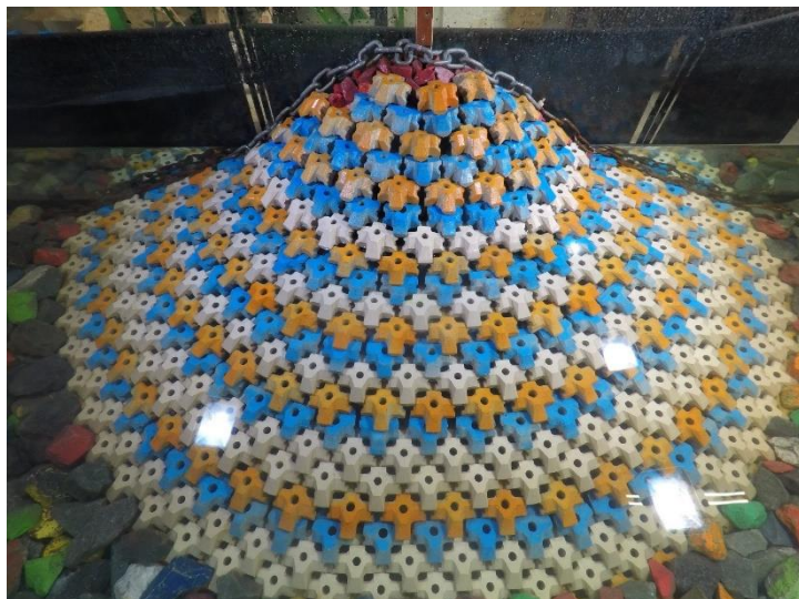
Figure D.34. Structure after 0.8 H_{m0} test run of Series 1.4.1 ( N_s = 1.93 ).
