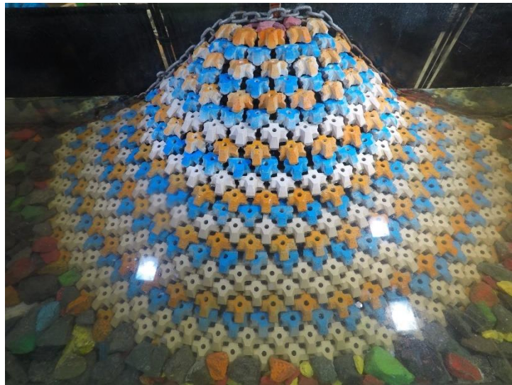
Figure D.1. Structure before 0.8 H_{m0} test run of Series 0.1.
