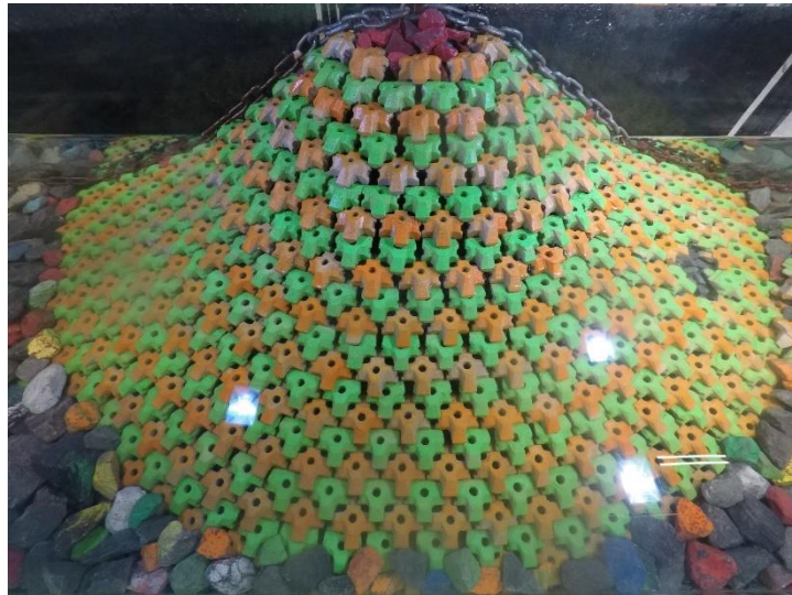
Figure D.56. Structure after 1.2 H_{m0} test run of Series 2.2 ( N_s = 2.97 ).
