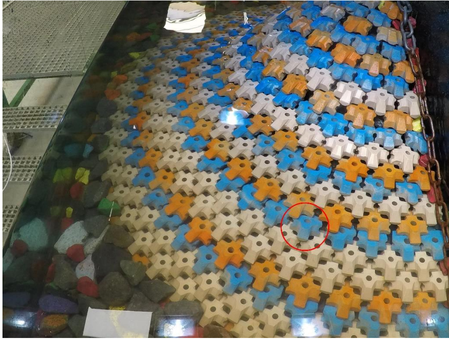
Figure 6.6. Unfavourable orientation of XP-Curve unit after Series 1.1.
