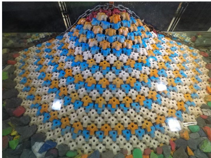
Figure D.42. Structure after 1.1 H_{m0} test run of Series 1.4.2 ( N_s = 2.72 ).
