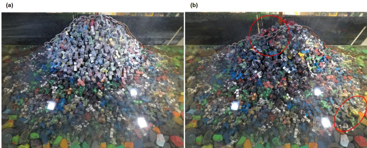
Figure 6.27. Xbloc model of Series 3.1 (a) before 0.6 H_{m0} test run and (b) after failure at 1.2 H_{m0} test run with settlements and extracted units indicated.
