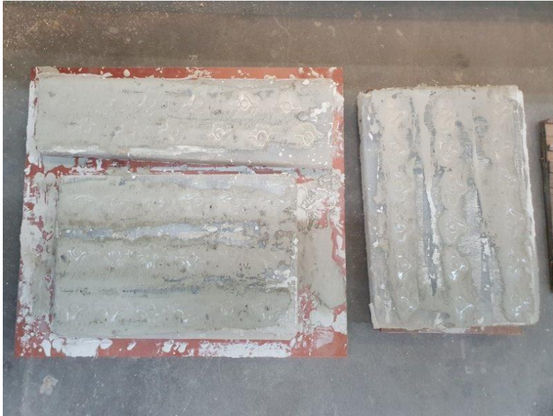
Figure B.3. Rubber moulds filled with mortar.
