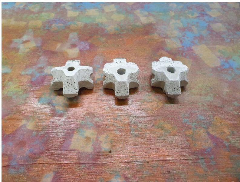
Figure B.4. The three distinct armour units after demoulding and polishing.
