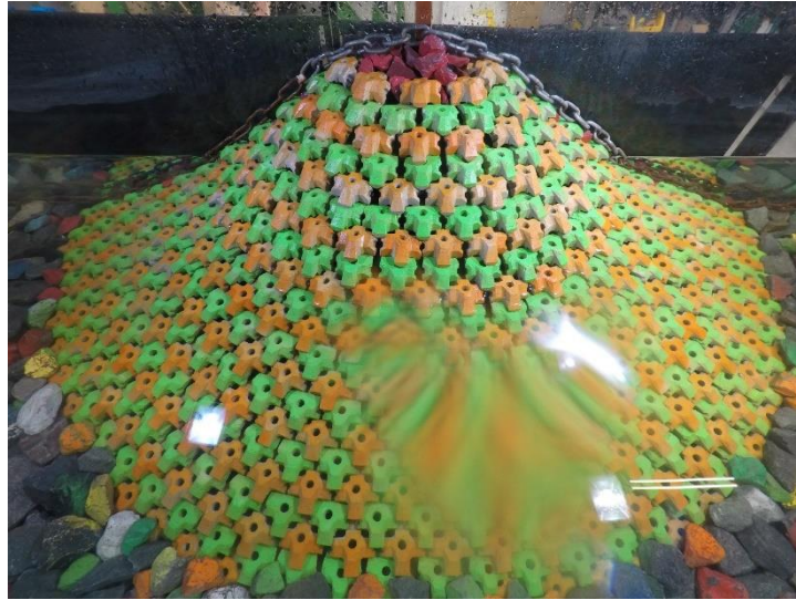
Figure D.46. Structure after 0.8 H_{m0} test run of Series 2.1 ( N_s = 1.95 ).
