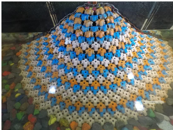
Figure D.11. Structure after 1.2 H_{m0} test run of Series 1.1 ( N_s = 2.87 ).
