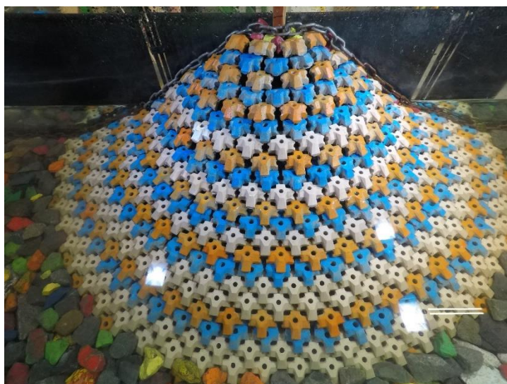
Figure D.18. Structure after 1.2 H_{m0} test run of Series 1.2.1 ( N_s = 3.09 ).
