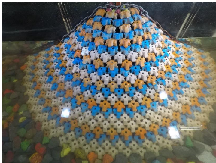
Figure D.9. Structure after 1.0 H_{m0} test run of Series 1.1 ( N_s = 2.56 ).
