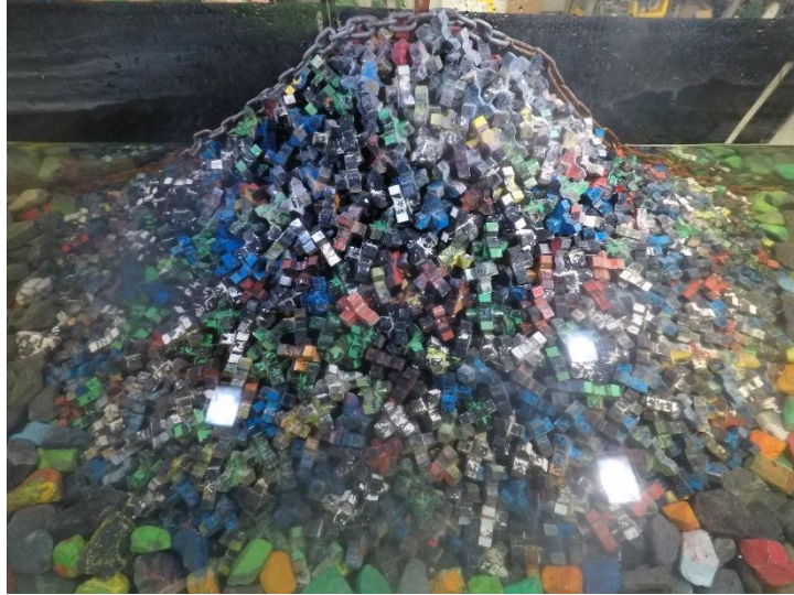
Figure D.71. Structure after 0.8 H_{m0} test run of Series 3.1 ( N_s = 2.00 ).
