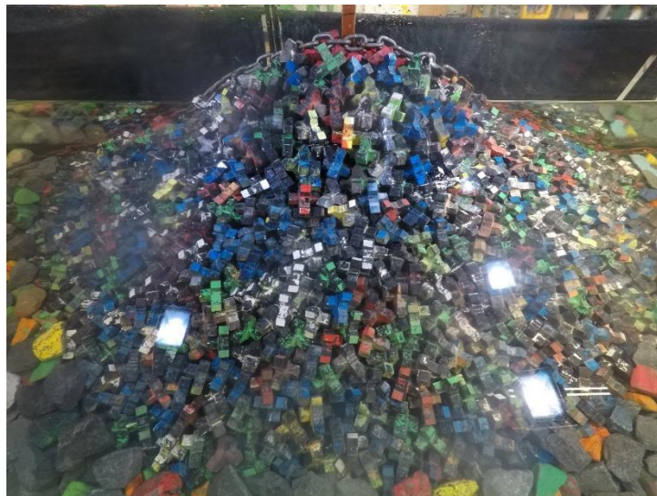
Figure D.81. Structure after 1.2 H_{m0} test run of Series 3.2 ( N_s = 3.14 ).
