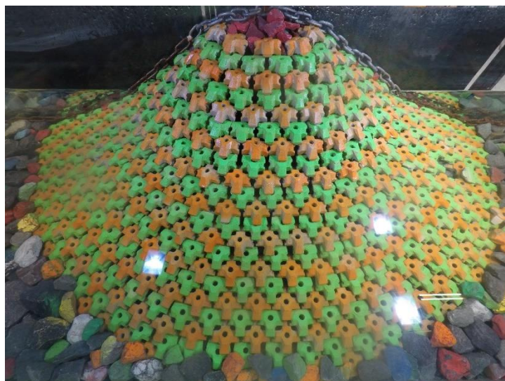
Figure D.54. Structure after 1.0 H_{m0} test run of Series 2.2 ( N_s = 2.50 ).
