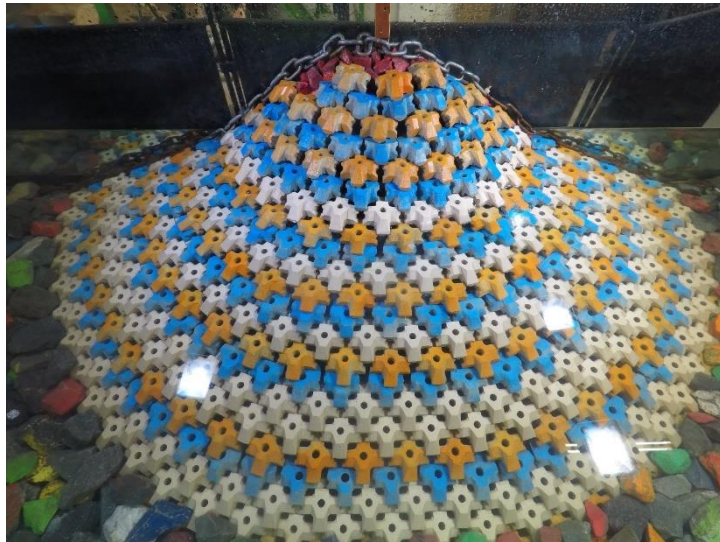
Figure D.36. Structure after 1.1 H_{m0} test run of Series 1.4.1 ( N_s = 2.71 ).
