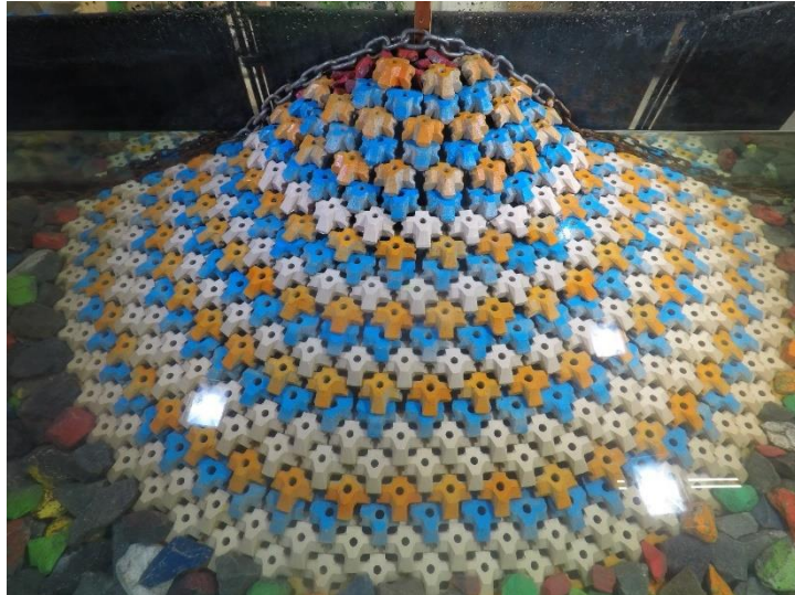
Figure D.32. Structure after 1.5 H_{m0} test run of Series 1.3 ( N_s = 3.23 ).
