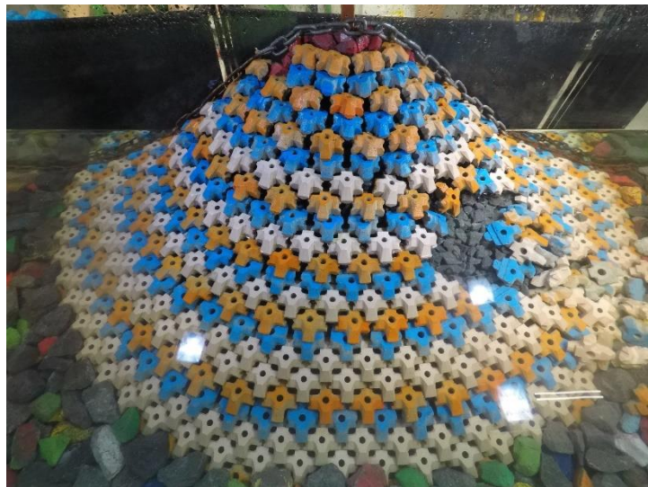
Figure D.24. Structure after 1.2 H_{m0} test run of Series 1.2.2 ( N_s = 3.01 ).
