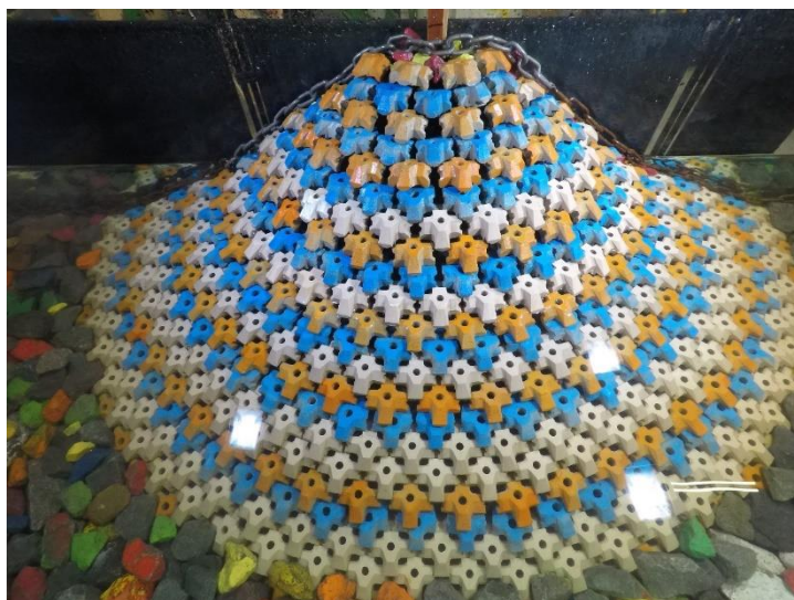
Figure D.16. Structure after 1.0 H_{m0} test run of Series 1.2.1 ( N_s = 2.60 ).
