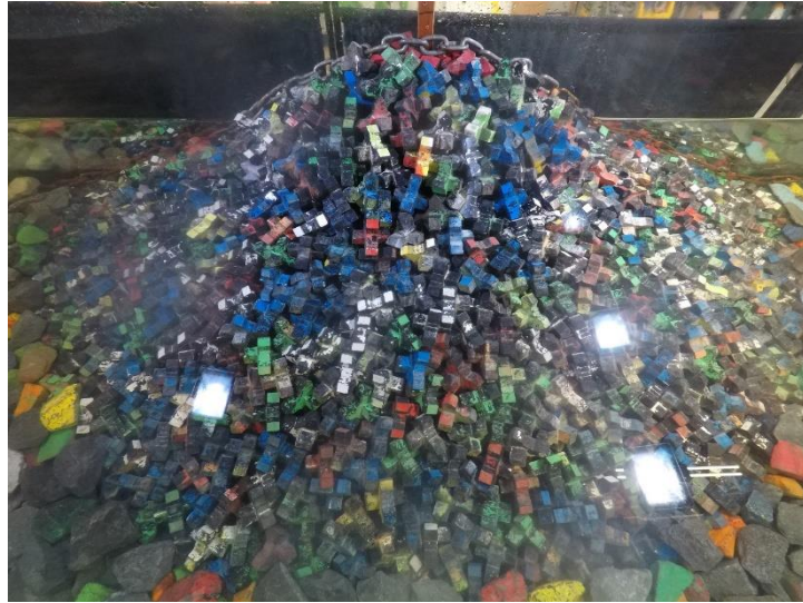
Figure D.80. Structure after 1.1 H_{m0} test run of Series 3.2 ( N_s = 2.77 ).
