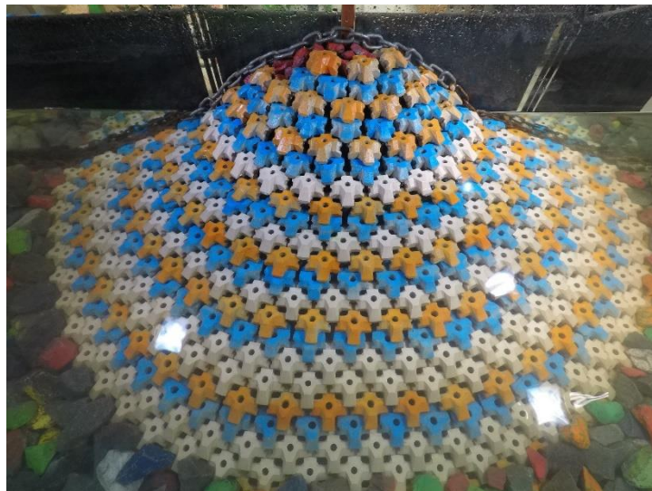
Figure D.27. Structure after 1.0 H_{m0} test run of Series 1.3 ( N_s = 2.60 ).
