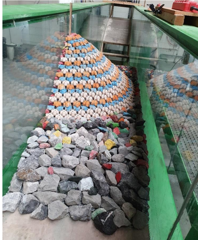
Figure 4.2. Toe structure applied in physical model.
