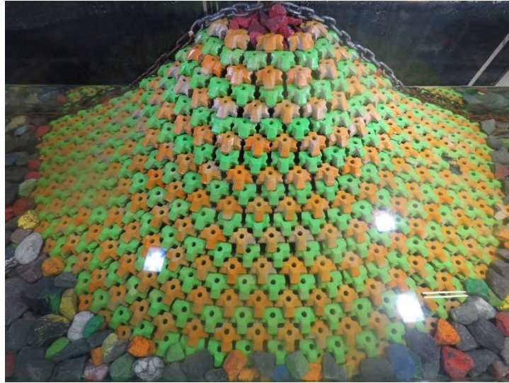
Figure D.55. Structure after 1.1 H_{m0} test run of Series 2.2 ( N_s = 2.74 ).
