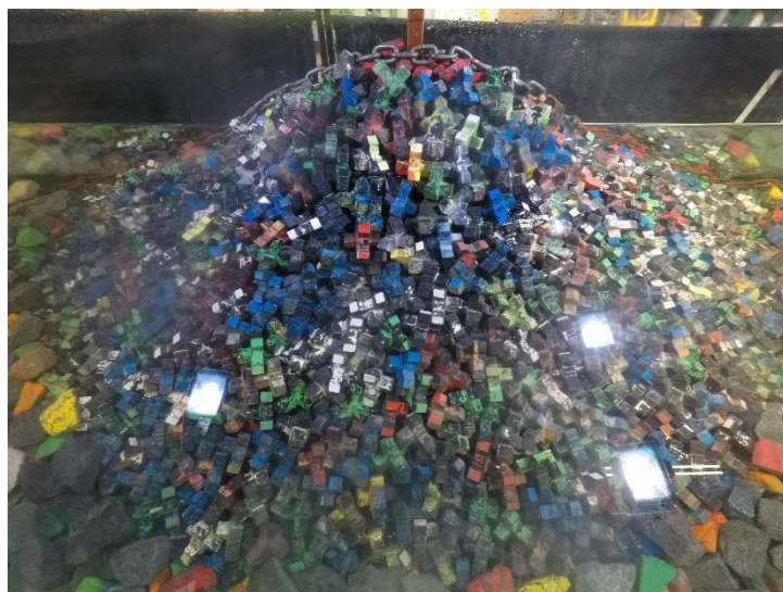
Figure D.82. Structure after 1.3 H_{m0} test run of Series 3.2 ( N_s = 3.34 ).
