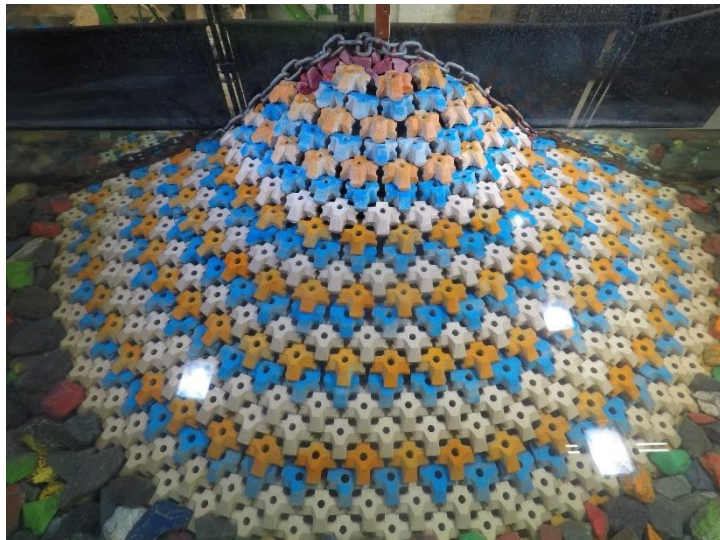
Figure D.33. Structure before 0.8 H_{m0} test run of Series 1.4.1.
