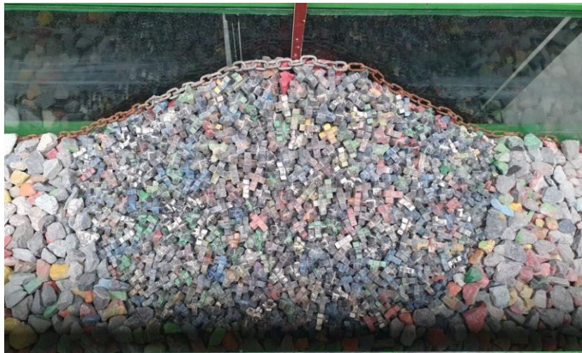
Figure 4.10. Top view of Xbloc model.
