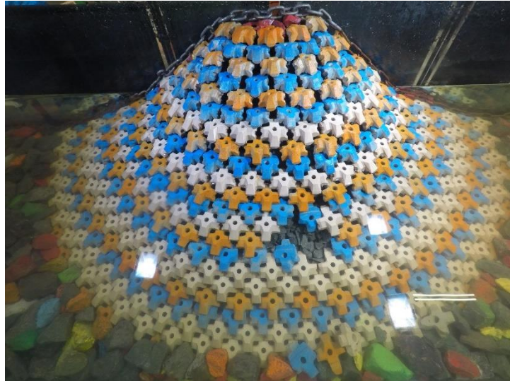
Figure D.6. Structure after 1.3 H_{m0} test run of Series 0.1 ( N_s = 3.28 ).
