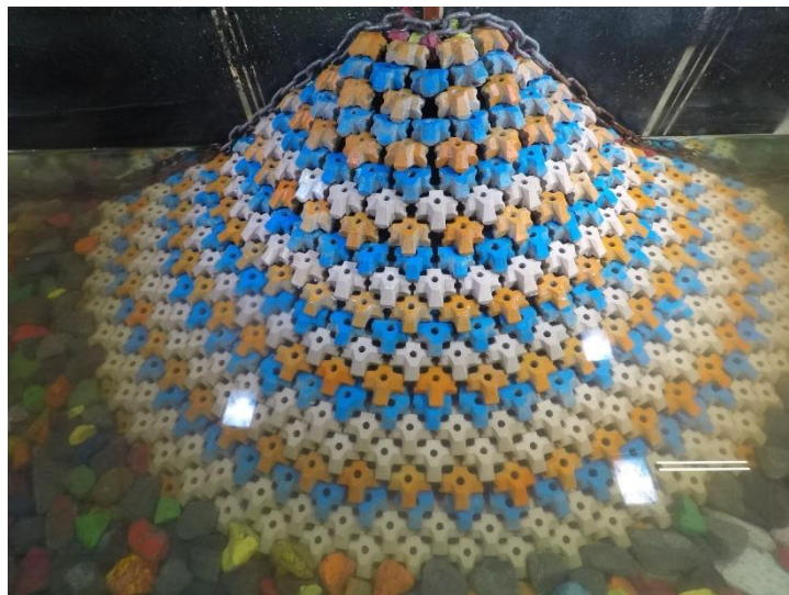
Figure D.8. Structure after 0.8 H_{m0} test run of Series 1.1 ( N_s = 1.82 ).
