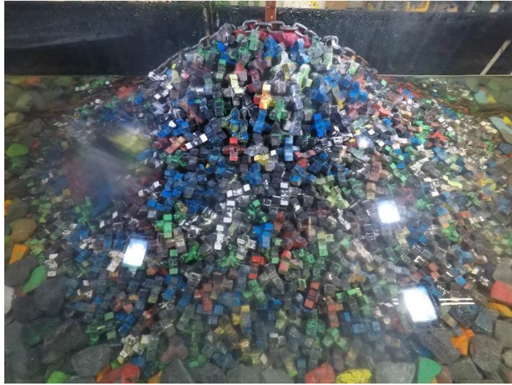
Figure D.77. Structure after 0.8 H_{m0} test run of Series 3.2 ( N_s = 2.00 ).
