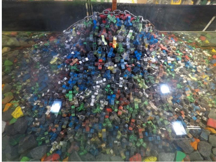
Figure D.83. Structure after 1.4 H_{m0} test run of Series 3.2 ( N_s = 3.45 ).
