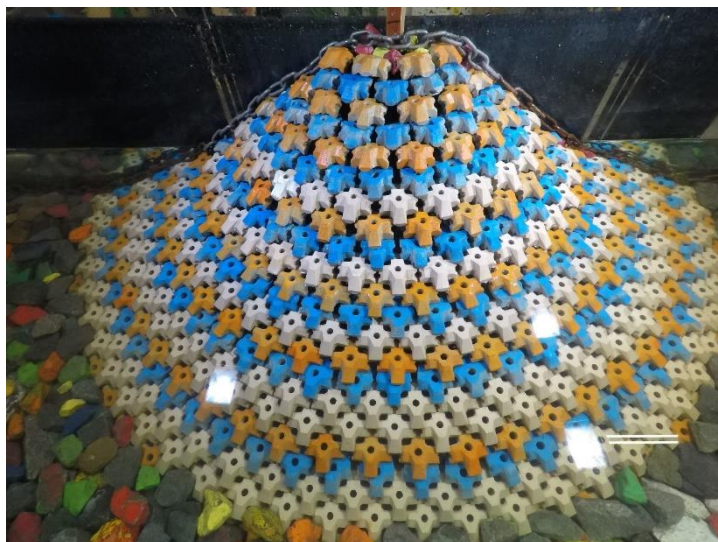
Figure D.15. Structure after 0.8 H_{m0} test run of Series 1.2.1 ( N_s = 2.38 ).
