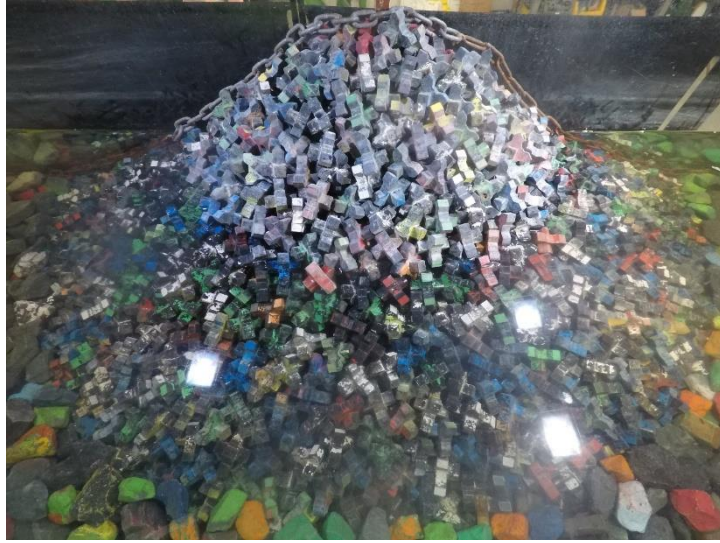
Figure D.69. Structure before 0.6 H_{m0} test run of Series 3.1.
