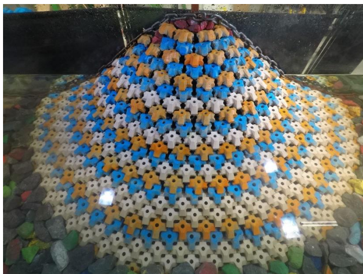
Figure D.22. Structure after 1.0 H_{m0} test run of Series 1.2.2 ( N_s = 2.47 ).
