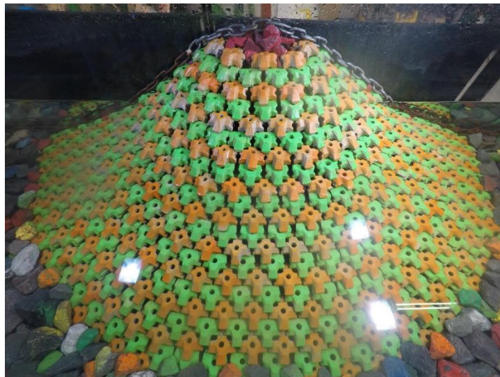
Figure D.50. Structure after 1.3 H_{m0} test run of Series 2.1 ( N_s = 3.26 ).
