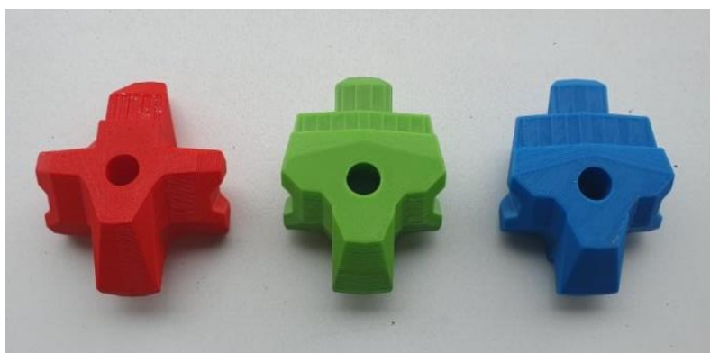
Figure B.1. Three-dimensional prints of the armour unit concepts.
