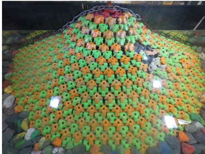
Figure D.68. Structure after 1.2 H_{m0} test run of Series 2.4 ( N_s = 2.90 ).
