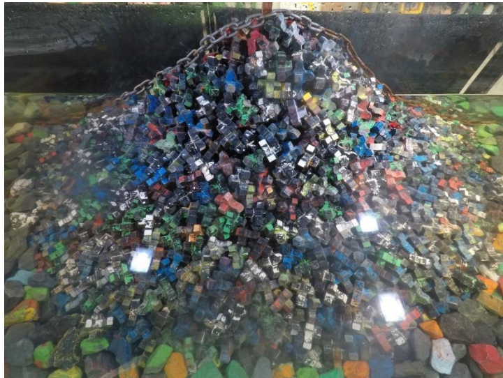
Figure D.72. Structure after 1.0 H_{m0} test run of Series 3.1 ( N_s = 2.50 ).
