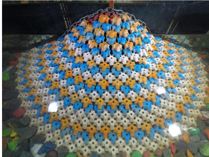
Figure D.29. Structure after 1.2 H_{m0} test run of Series 1.3 ( N_s = 2.88 ).
