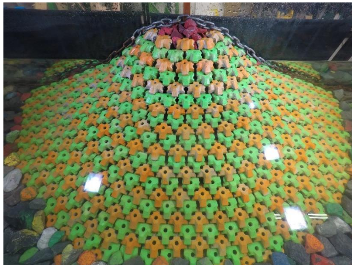
Figure D.59. Structure after 1.0 H_{m0} test run of Series 2.3 ( N_s = 2.60 ).
