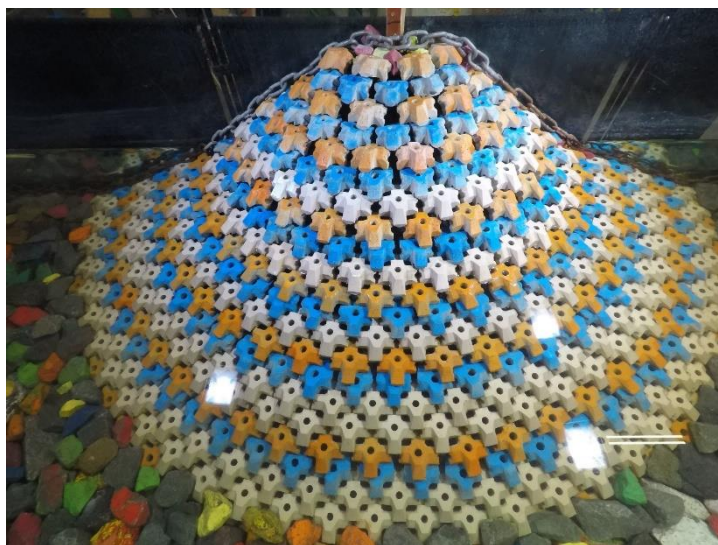
Figure D.14. Structure before 0.8 H_{m0} test run of Series 1.2.1.
