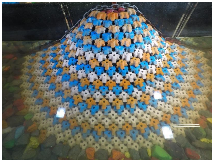
Figure D.3. Structure after 1.0 H_{m0} test run of Series 0.1 ( N_s = 2.64 ).
