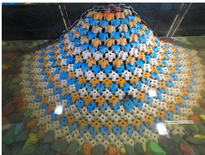
Figure D.4. Structure after 1.1 H_{m0} test run of Series 0.1 ( N_s = 2.81 ).
