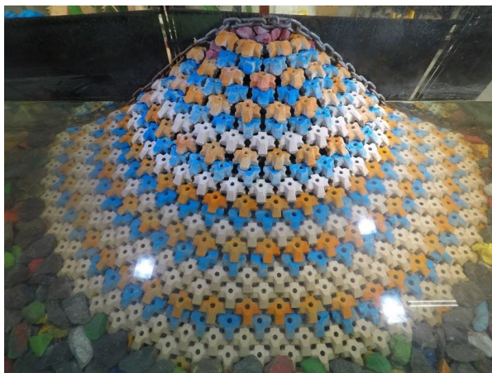
Figure D.20. Structure before 0.8 H_{m0} test run of Series 1.2.2.
