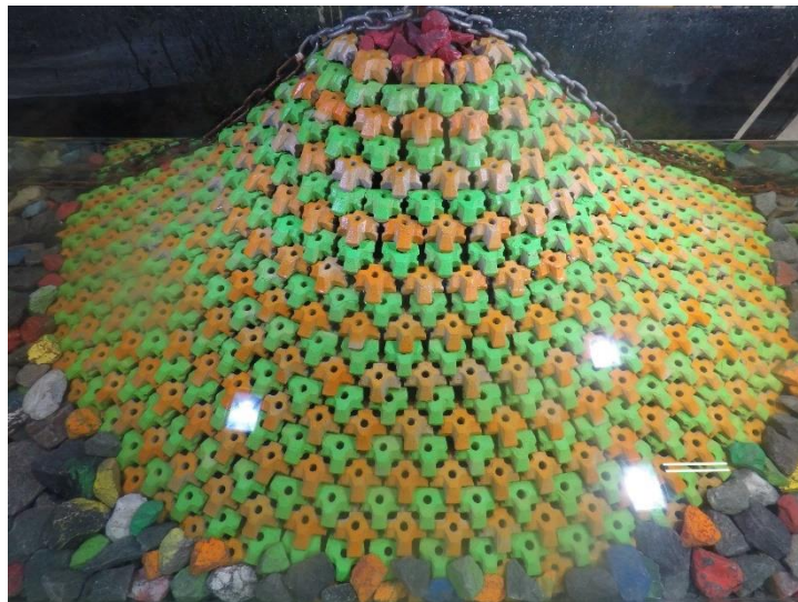
Figure D.53. Structure after 0.8 H_{m0} test run of Series 2.2 ( N_s \approx 1.96 ).
