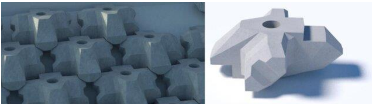
Figure 2.9. XblocPlus placement pattern (left) and side view of unit (right) (Reedijk et al., 2018).
