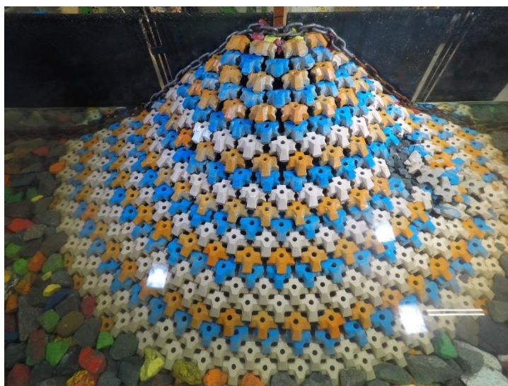
Figure D.19. Structure after 1.3 H_{m0} test run of Series 1.2.1 ( N_s = 4.04 ).
