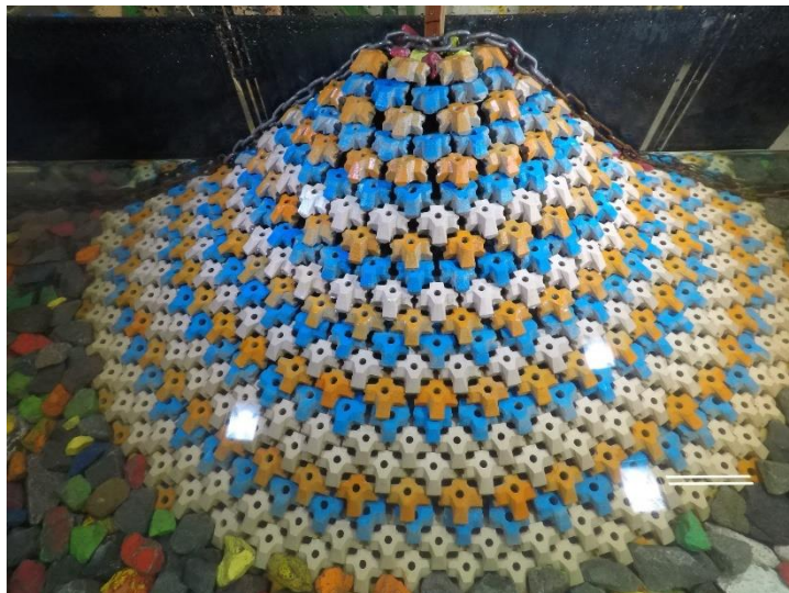
Figure D.17. Structure after 1.1 H_{m0} test run of Series 1.2.1 ( N_s = 2.70 ).
