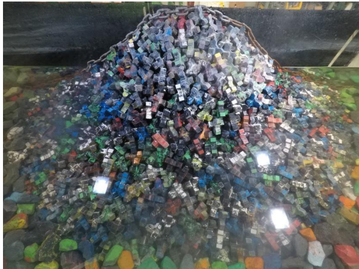
Figure D.70. Structure after 0.6 H_{m0} test run of Series 3.1 ( N_s = 1.41 ).
