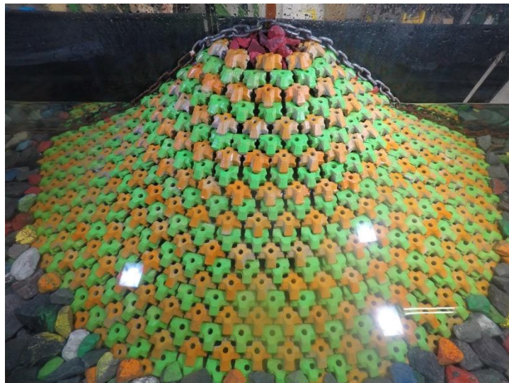
Figure D.47. Structure after 1.0 H_{m0} test run of Series 2.1 ( N_s = 2.45 ).
