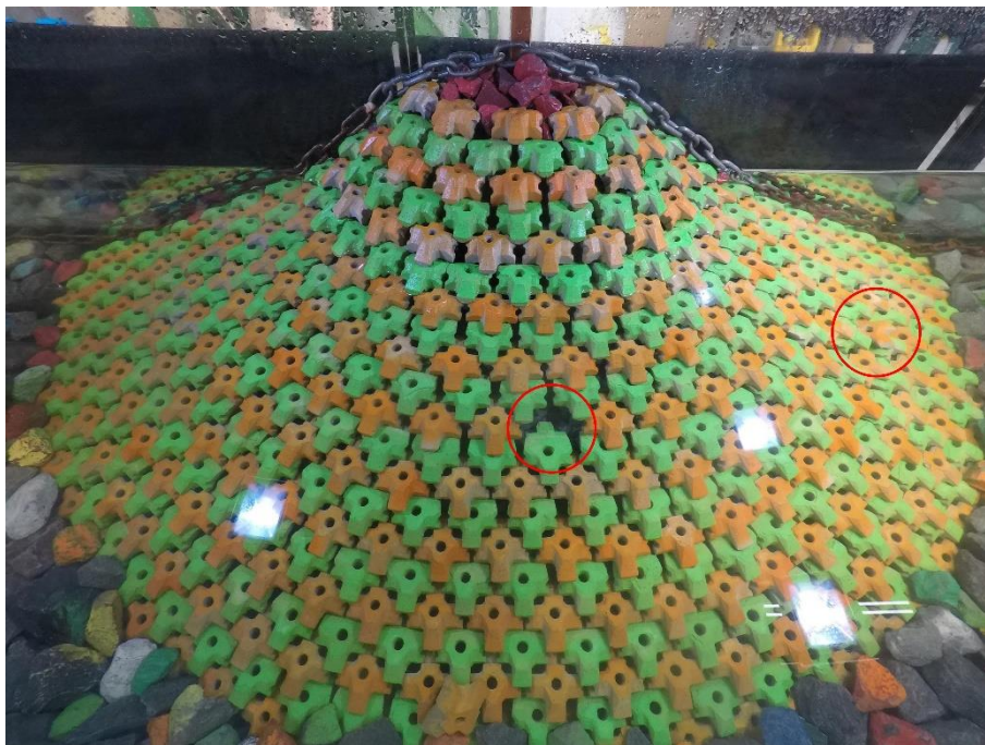
Figure 7.2. Rotation out of the armour layer of two individual column-positioned XP-Base units during Series 2.3.
