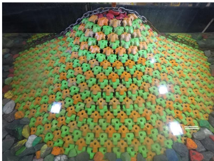
Figure D.66. Structure after 1.0 H_{m0} test run of Series 2.4 ( N_s = 2.52 ).
