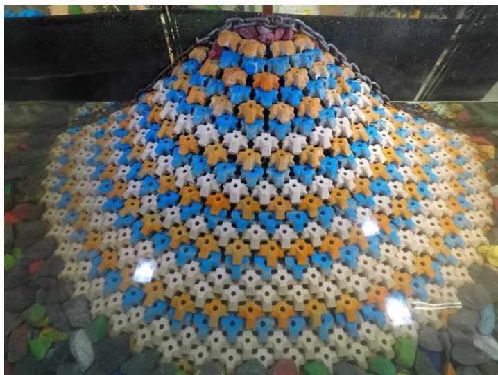
Figure D.21. Structure after 0.8 H_{m0} test run of Series 1.2.2 ( N_s = 1.96 ).
