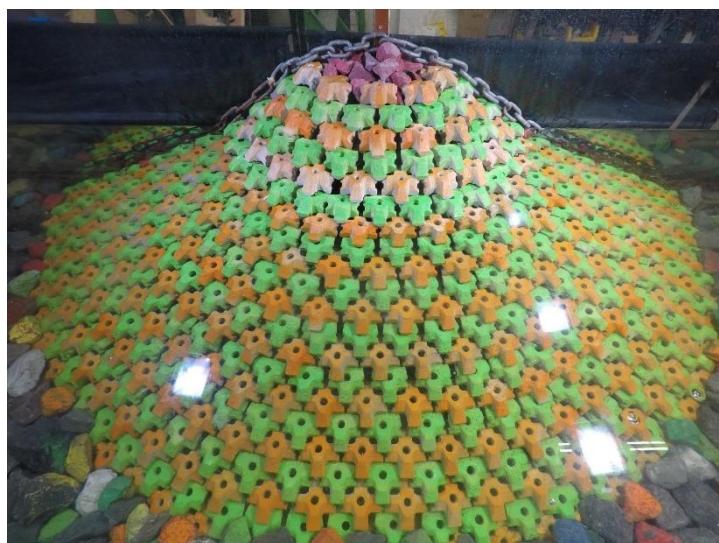
Figure D.57. Structure before 0.8 H_{m0} test run of Series 2.3.
