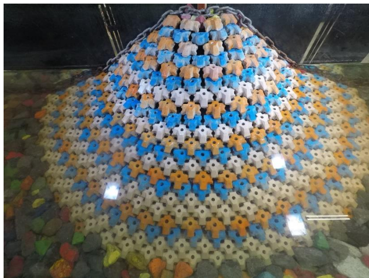
Figure D.7. Structure before 0.8 H_{m0} test run of Series 1.1.
