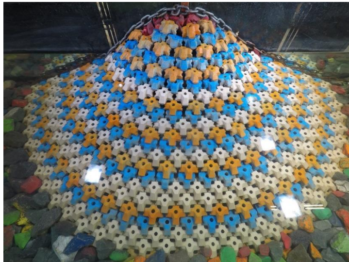
Figure D.39. Structure before 0.8 H_{m0} test run of Series 1.4.2.
