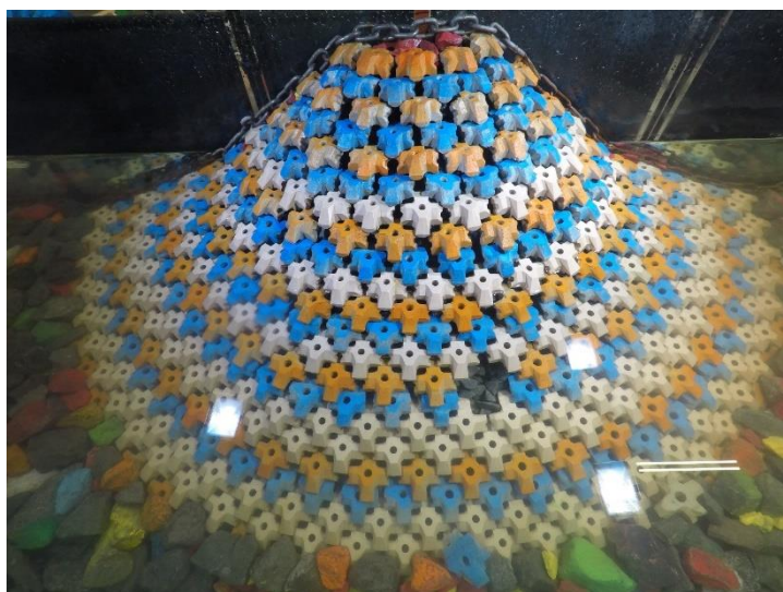
Figure D.5. Structure after 1.2 H_{m0} test run of Series 0.1 ( N_s = 2.94 ).
