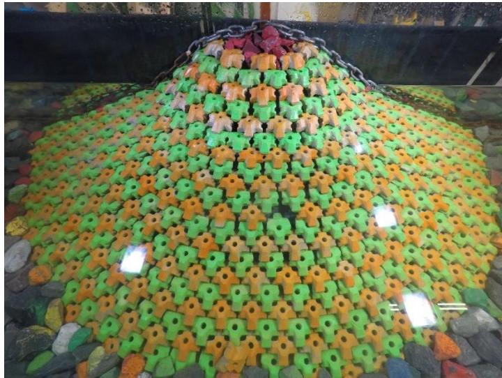
Figure D.62. Structure after 1.3 H_{m0} test run of Series 2.3 ( N_s = 3.18 ).
