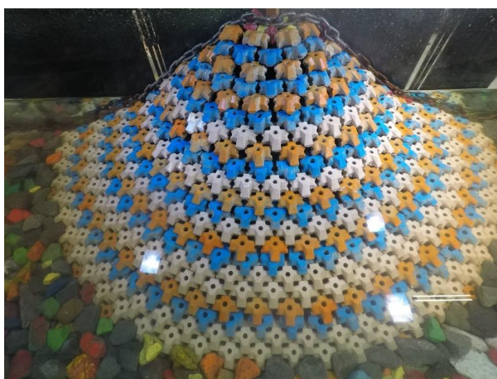
Figure D.13. Structure after 1.4 H_{m0} test run of Series 1.1 ( N_s = 3.38 ).
