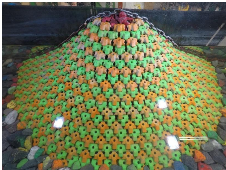
Figure D.45. Structure before 0.8 H_{m0} test run of Series 2.1.
