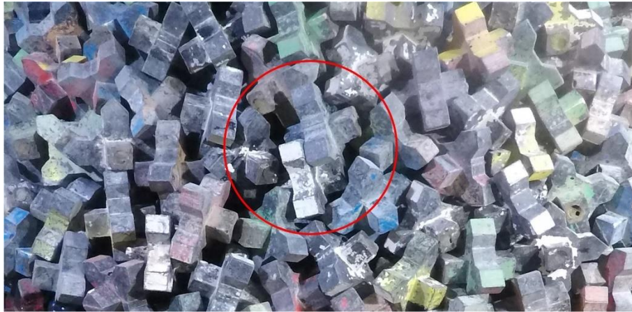
Figure 7.1. Unfavourable orientation of two Xbloc units due to a lack of randomness in placement in Series 3.1.
