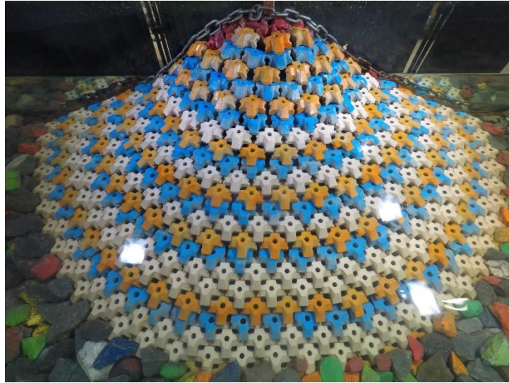
Figure D.41. Structure after 1.0 H_{m0} test run of Series 1.4.2 ( N_s = 2.58 ).
