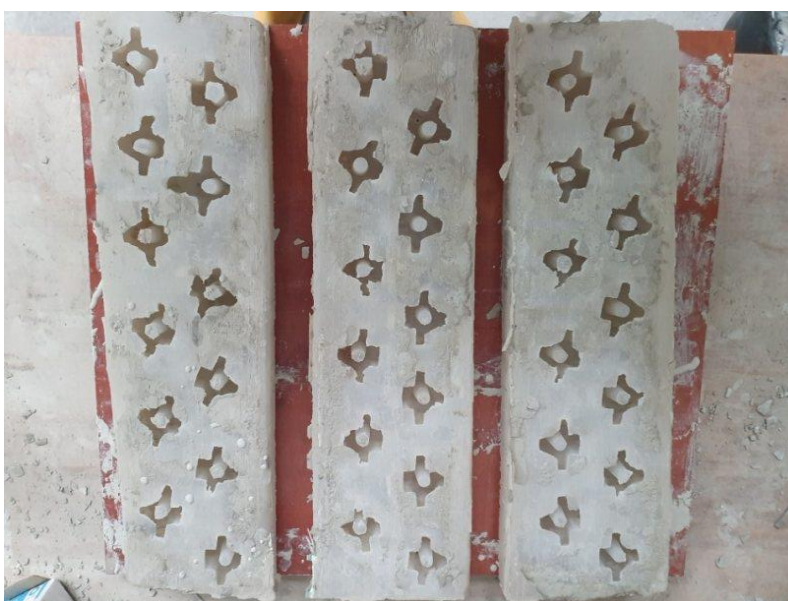
Figure B.2. Casting rubber moulds for the production of concrete armour units.
