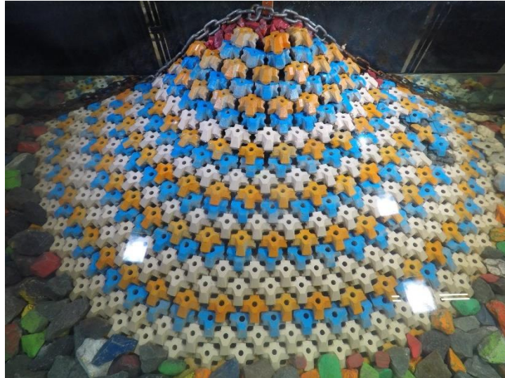
Figure D.44. Structure after 1.3 H_{m0} test run of Series 1.4.2 ( N_s = 3.14 ).
