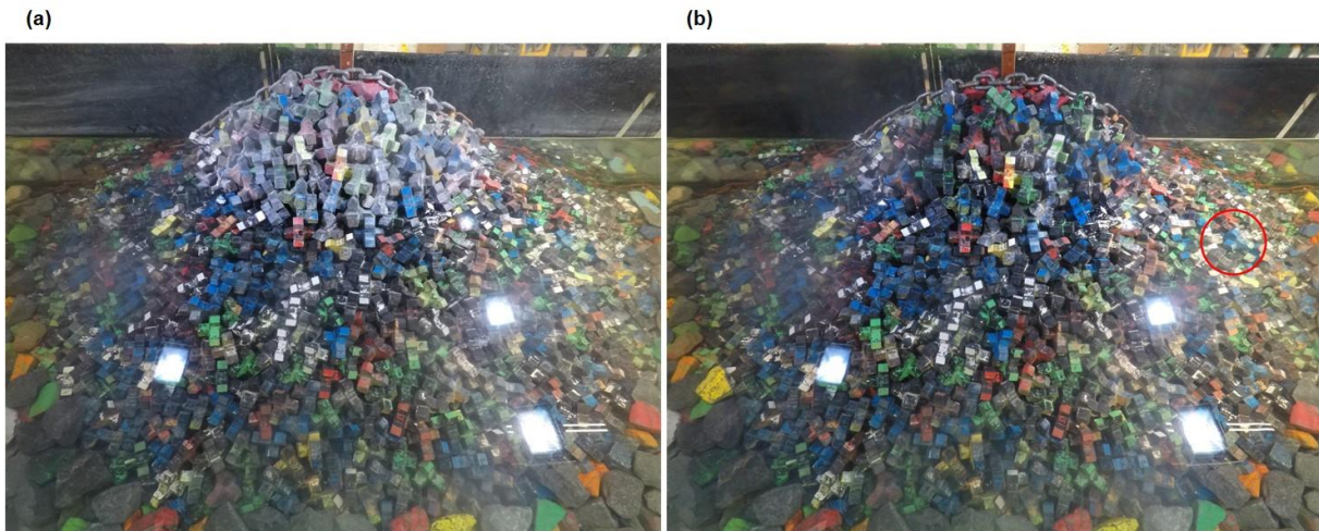
Figure 6.29. Xbloc model of Series 3.2 (a) before 0.6 H_{m0} test run and (b) after failure at 1.2 H_{m0} test run with extracted unit indicated.
