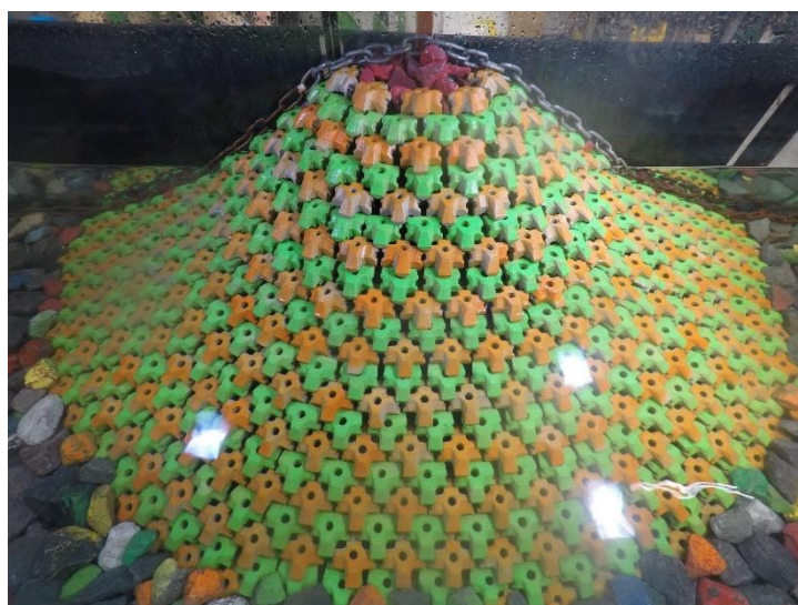
Figure D.51. Structure after 1.4 H_{m0} test run of Series 2.1 ( N_s = 3.31 ).
