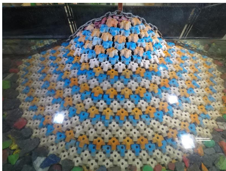
Figure D.25. Structure before 0.8 H_{m0} test run of Series 1.3.
