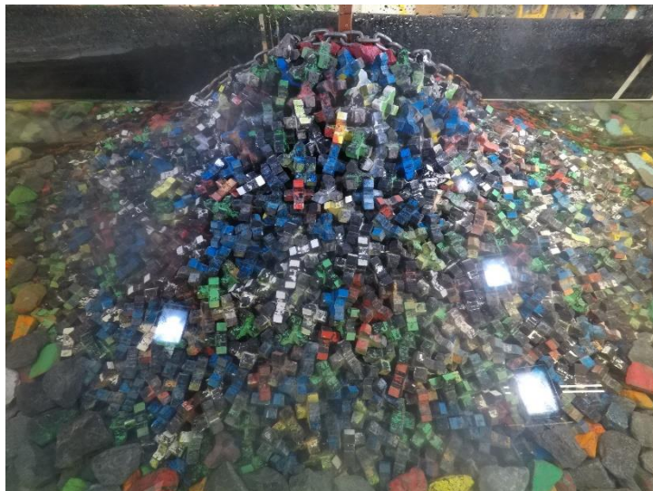
Figure D.78. Structure after 0.9 H_{m0} test run of Series 3.2 ( N_s = 2.32 ).
