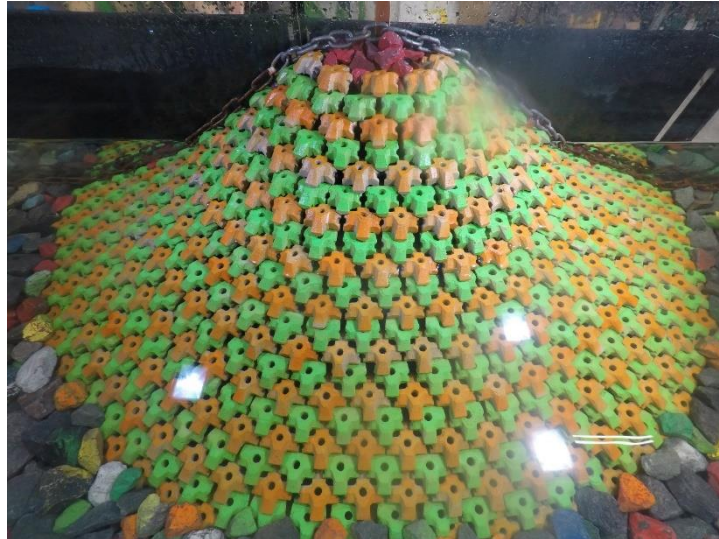
Figure D.49. Structure after 1.2 H_{m0} test run of Series 2.1 ( N_s = 2.92 ).
