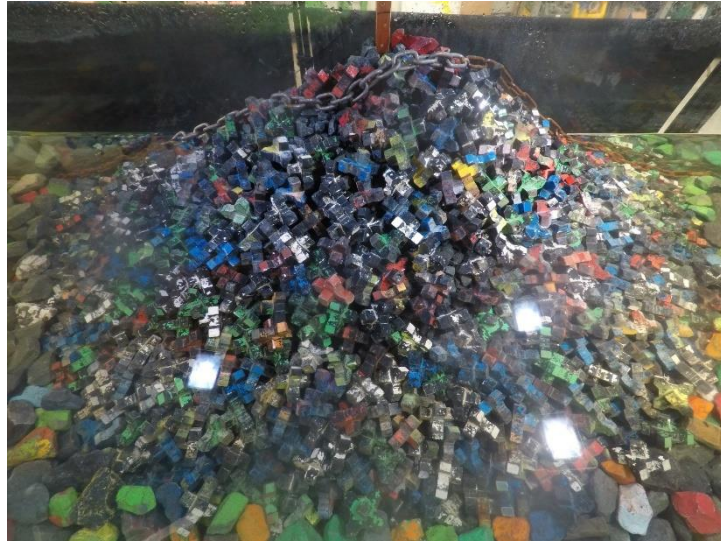
Figure D.74. Structure after 1.2 H_{m0} test run of Series 3.1 ( N_s = 2.99 ).
