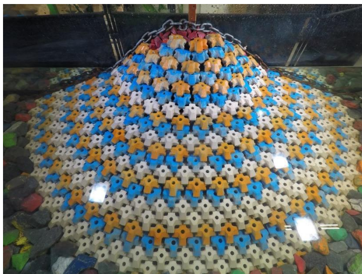
Figure D.37. Structure after 1.2 H_{m0} test run of Series 1.4.1 ( N_s = 2.91 ).
