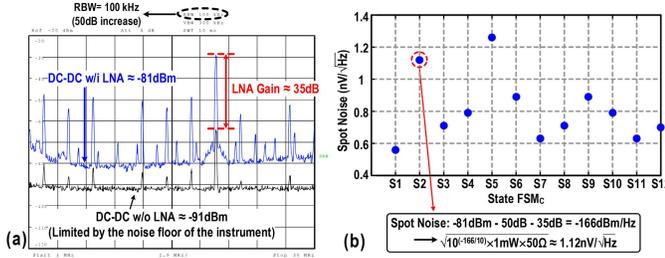
Fig. 19. (a) Spectrum of the output voltage of the DC-DC converter with (blue line) and without (black line) the use of an LNA; (b) spot noise of the converter across different FSM<sub>C</sub> state.
