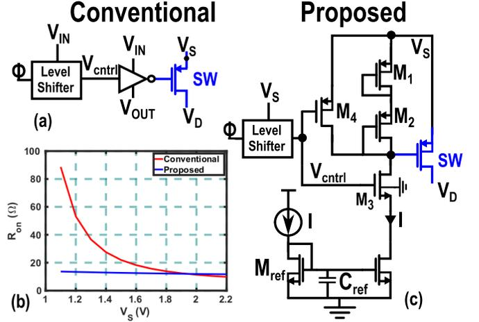
Fig. 9. (a) Schematic of a conventional gate-driver circuit, with (b) the equivalent series resistance versus the supply voltage, and (c) the proposed gate driver circuit, resulting in a constant  $R_{on}$ .
