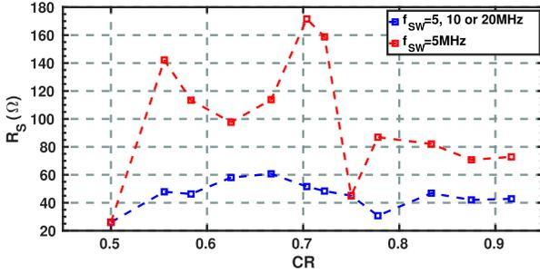
Fig. 5. Calculated output resistance of the converter with fixed (red) and adaptive (blue) switching frequency.
