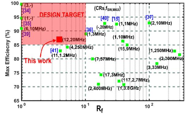
Fig. 20. Peak power efficiency of state-of-the-art DC-DC converters versus the ratio of maximum-to-minimum switching frequency ( $R_f = \frac{f_{SW,max}}{f_{SW,min}}$ ). The number of implemented CRs, and  $f_{SW,max}$  are reported in the parenthesis.
