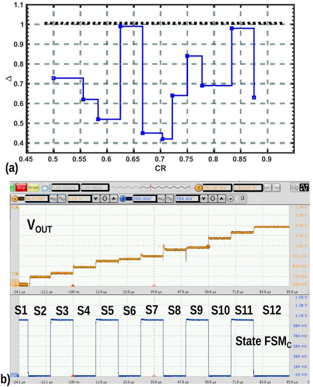
Fig. 16. Measurement results of (a) the resolution of the converter for  $V_{IN} = V_{INmax} = 2.2\text{ V}$  and  $I_L = I_{Lmin} = 0.5\text{ mA}$ ; (b) the monotonicity of the converter for  $V_{IN} = V_{INmin} = 1.3\text{ V}$  and  $I_L = I_{Lmax} = 2\text{ mA}$ .
