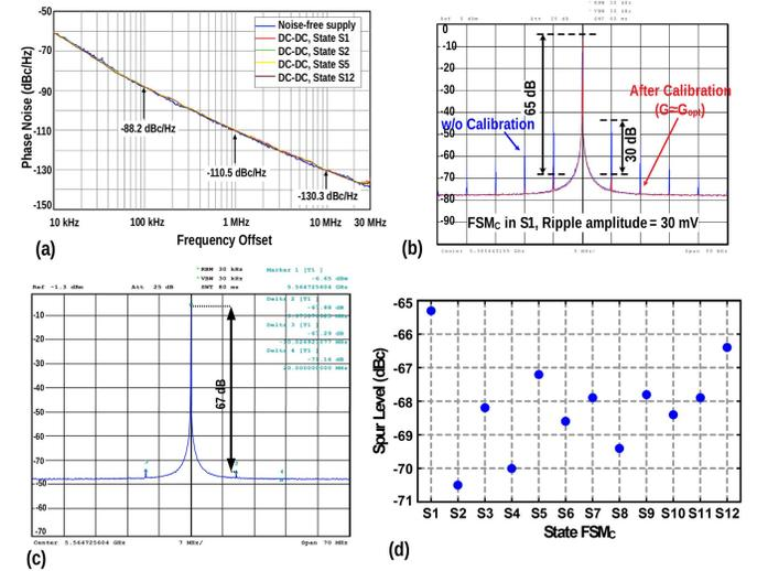
Fig. 21. (a) Measured oscillator PN performance at  $f = 5.5 \text{ GHz}$  and (b) its spectrum before and after calibration of the SRB with FSM<sub>C</sub> in State S1 and (c) State S5; (d) spur level across different converter states when the oscillator is calibrated only at State S1.
