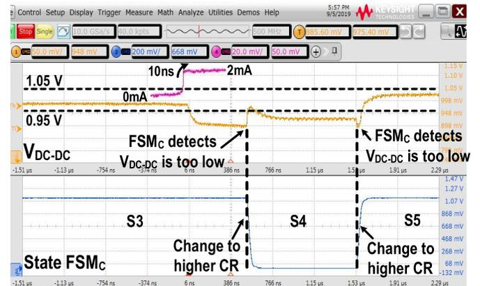
Fig. 18. Response of the converter (orange line) to a current step from 0–2 mA (purple line) along with the signal that triggers the change in the FSM<sub>C</sub> (blue line).
