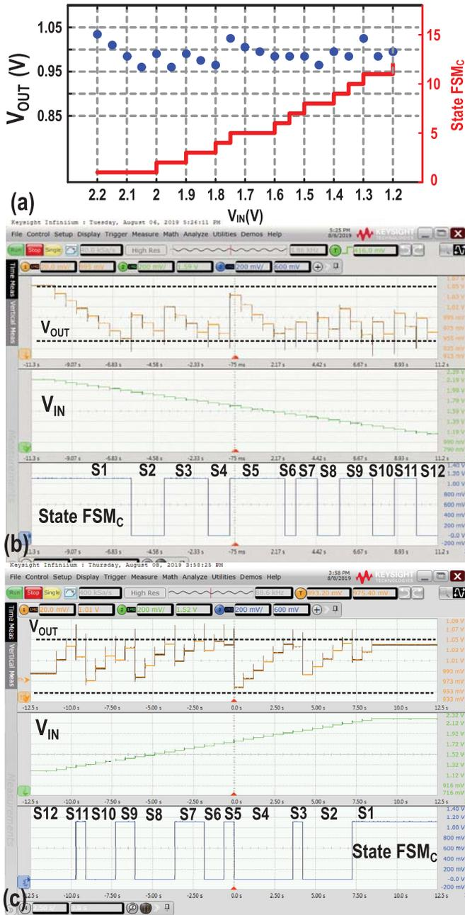
Fig. 15. (a) Measured output voltage of the DC-DC converter versus  $V_{IN}$  for  $I_L = 1\text{ mA}$ ; (b) transient waveform of  $V_{OUT}$  for descending and (c) ascending  $V_{IN}$  values along with the signal, that triggers the change in the FSM.
