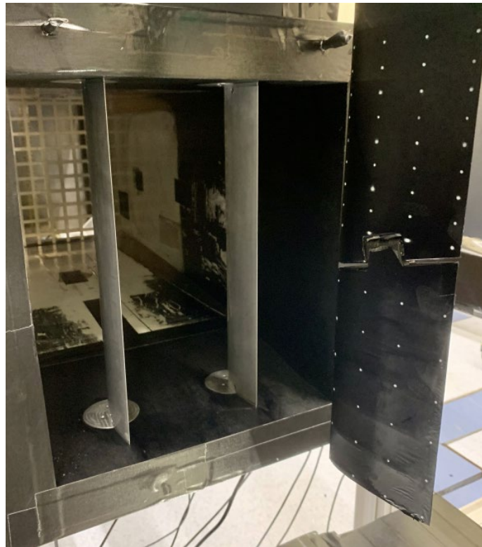
Figure 2: Wing model with folding wingtip mounted vertically in the test section, with an upstream view of the gust generator and the turbulence grid inside the wind tunnel nozzle.
