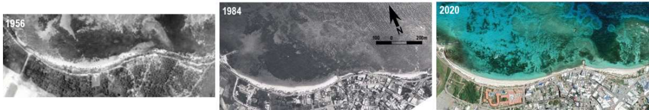
Figure 2.36: Shore line of Spratt Bight over the past 60 years (Martín-Prieto, et al., 2013).
