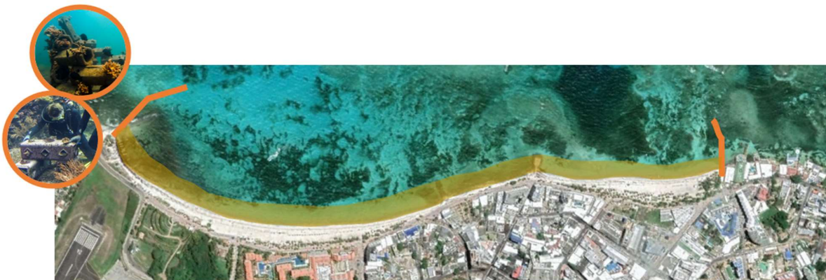
Figure 5.7: Impression of location for breakwaters in order to avoid sediment losses due to longshore transport after nourishment. On the left examples of artificial coral reefs.
