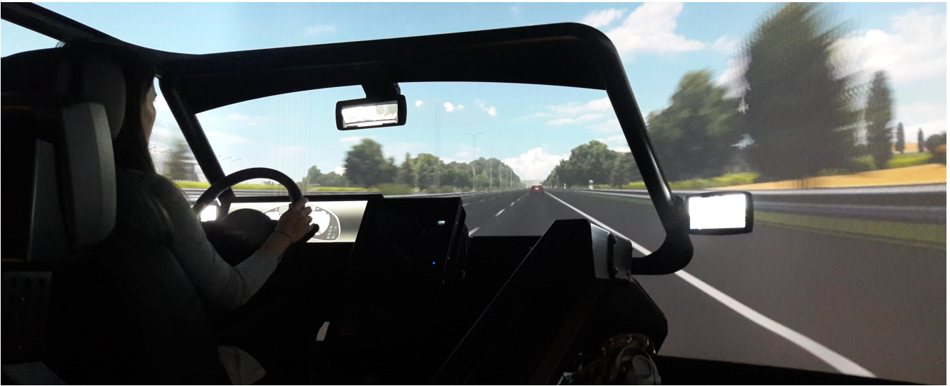
Fig. 1. The Cruden 6 degrees of freedom (6DoF) motion base driving simulator as used in the experiment, with actuated steering wheel, 210 degrees projection with side- and rear-view mirrors mounted to the a-pillars and windscreen frame.
