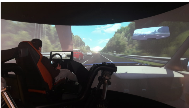
Figure 1: The Cruden motion base driving simulator as used in the experiment with actuated steering wheel and 210 degrees projection screen with on-screen side- and rearview mirrors.
