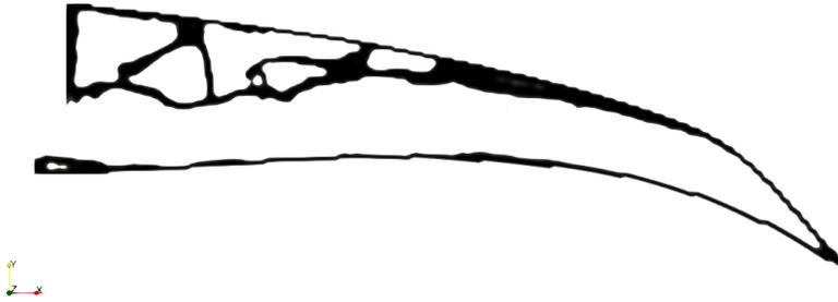
Figure 4.9: The expected deformed profile of the optimized trailing edge for  $x_{\min} = 1e - 9$ . Note the deformation is scaled from the linear analysis.
