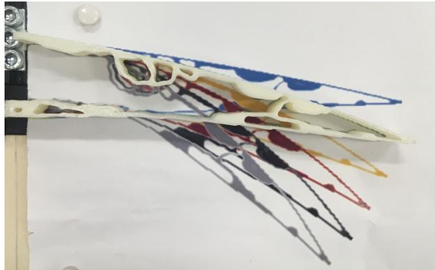
Figure 5.2: The prototype deformed according to the green profile, with an angle of  $6^\circ$  with respect to the neutral camber line.
