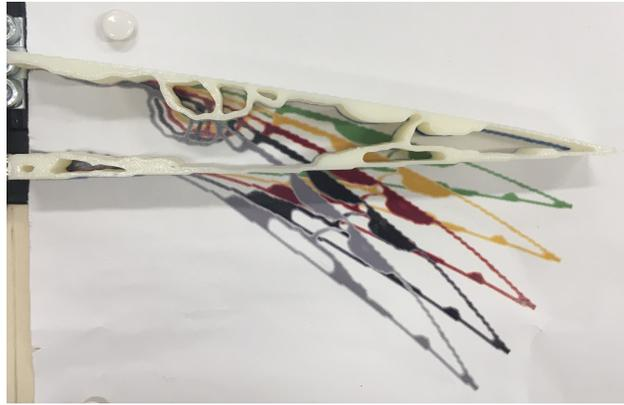
Figure 5.1: The set-up for testing the predicted output shape. The 3D printed model is fixed on the top left corner. The bottom left is fixed to a slider which slides through a metal profile. Behind the prototype, a print out of expected output shapes is attached for different degrees of deformation.
