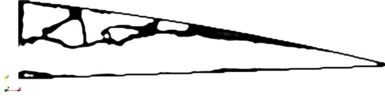
(a) The obtained structure from the optimization with  $x_{\min} = 0.001$ .
