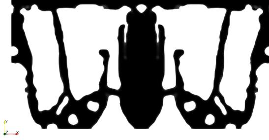
Figure 3.6: The shape adaptable mechanism obtained for 2 different inputs and outputs as defined in Fig. 3.3, for the dot product objective
