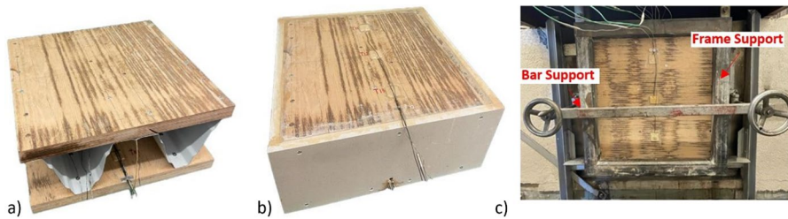
Fig. 4 WSH slab specimen: a WSH specimen after assembly, b WSH specimen after side insulation, c specimen mounting system
