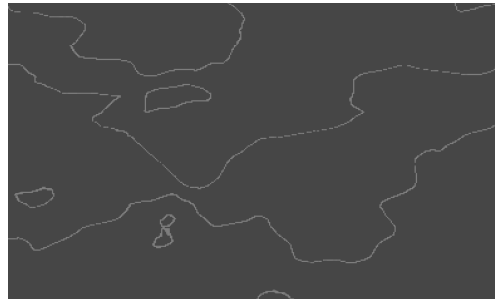
Figure 18: The caustic texture with correct alpha values. The grey background is the sky box, which means that the black parts seen in Figure 17 are now transparent.
