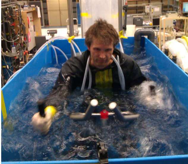
Figure 2: Sweat exercise in preconditioned tank on submerged cross-trainer
