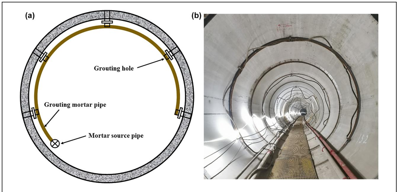
Figure 9. (a) Grouting holes of the segment and (b) inner structure.
