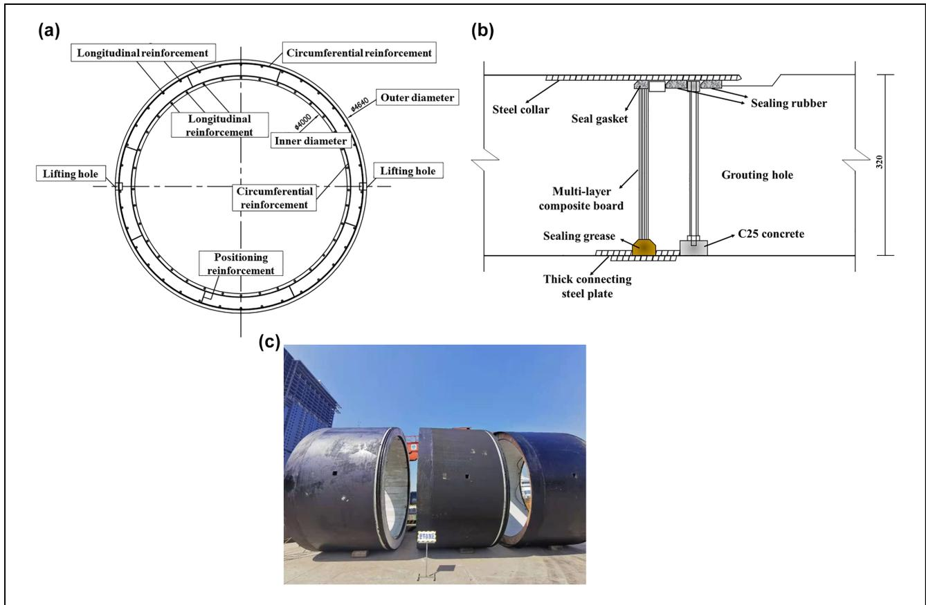
**Figure 6.** Segmental ring design: (a) segment cross-section, (b) segmental joint, and (c) precast segment with waterproof coating.
