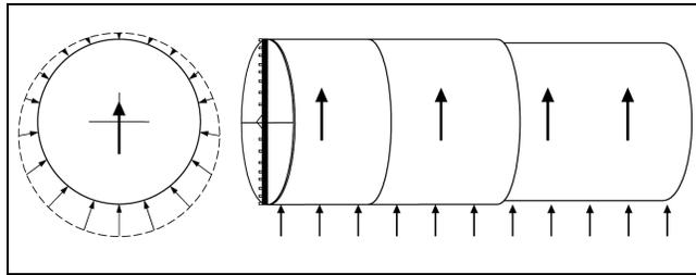
**Figure 12.** Uplift deviation of pipe jacking.
