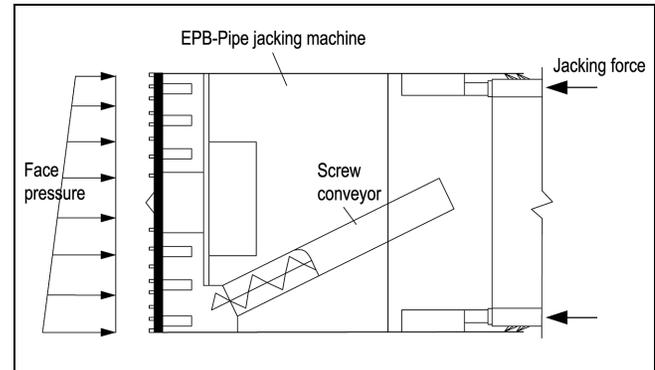
**Figure 7.** Face stability of earth pressure balance (EPB) pipe-jacking machine.
