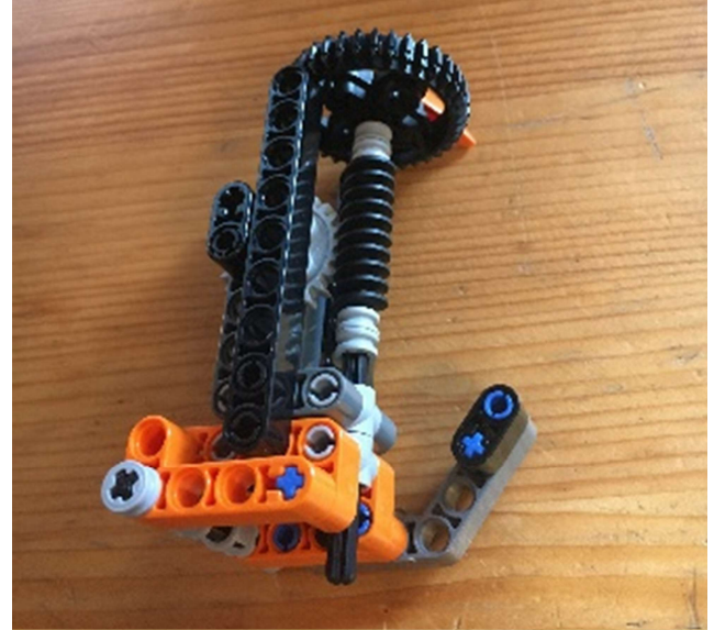
Figure 50: Screw mechanism build in LEGO.
