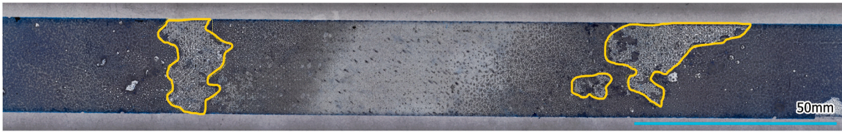
Fig. 6. Example of cohesive failure areas (highlighted) for BioPU Specimen 1.
