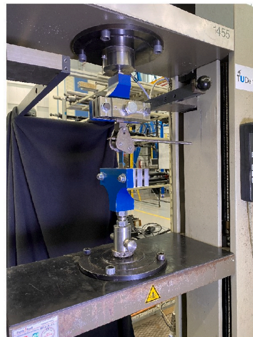
Fig. 5. a) Scheme of Floating roller peel test [33], b) Experimental set-up for floating roller peel tests.
