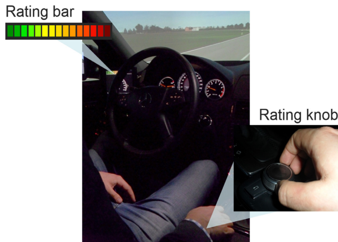
Fig. 2. Location of rating bar and rating knob in the car cabin. The rating bar has 15 coloured marks, where green/red marks indicated low/high perceived mismatch. (For interpretation of the references to colour in this figure legend, the reader is referred to the web version of this article.)
