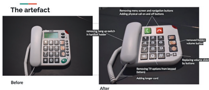
Image 16.6 Picture memory phone before and after modifications
