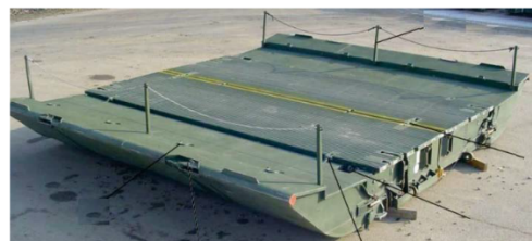
Figure 5. Floating pontoon bridge which is here proposed as BresDefender
