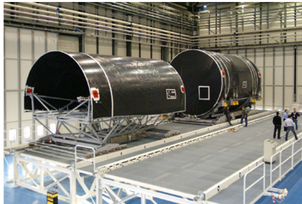
Figure 12.9: The upper fuselage part as it is mounted during production. [21]
