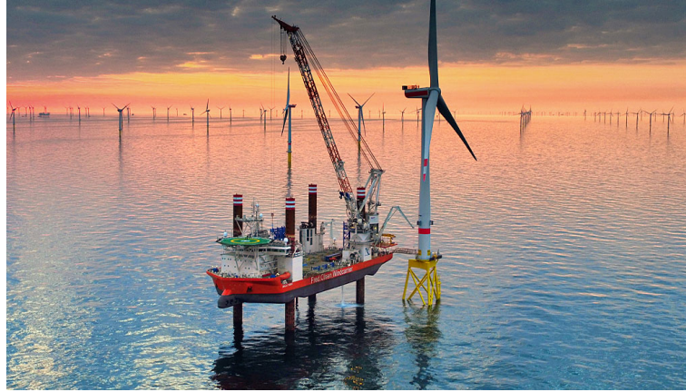
Figure 1.2: Typical Wind Turbine Installation Vessel (DNV , 2021).
