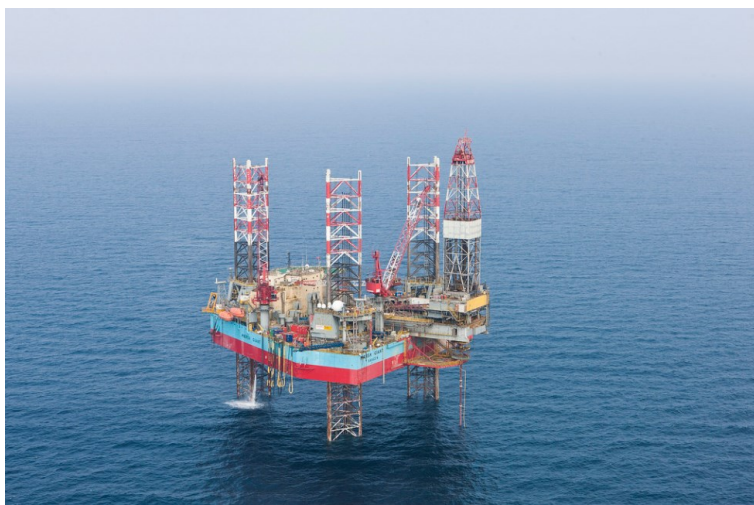
Figure 1.1: Typical self-elevating unit used for oil and gas exploration (M. J. Cassidy, 2011).
