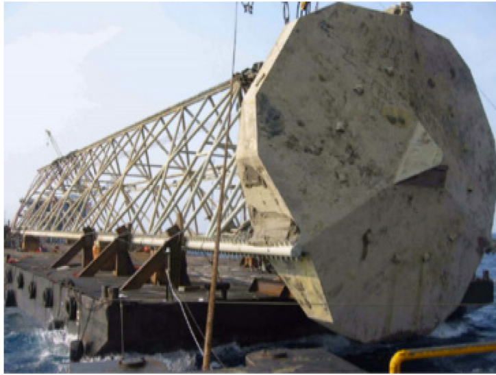
Figure 2.1: View of the spudcan's underside (Yi & Park, 2023).
