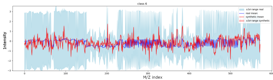
Figure 6-3: Visualization of the distribution of a single class, in blue mean and standard deviation of the original data and in red the mean and standard deviation of the generated data.
