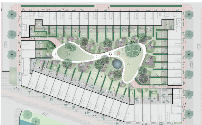
Figure 27: Ground floor plan, showing the shared garden in the centre, with the greenhouse as centerpiece. Shared amenities are situated near entrances (Delva Landsape Architectuur)
