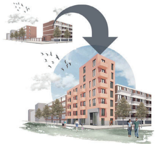
Figure 107: Example of adding housing on the blind facades in corners of portico flats (KAW architecten)
