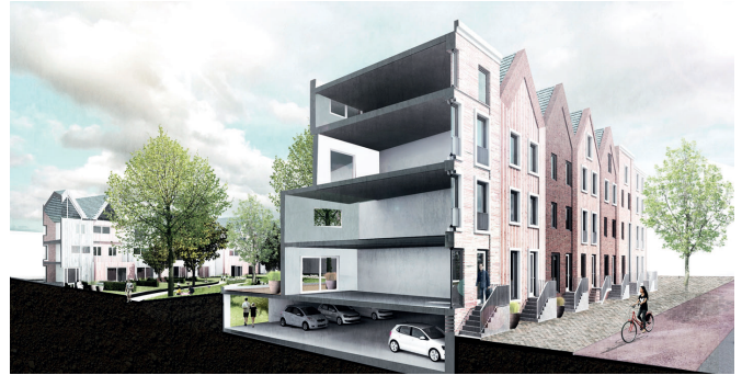
Figure 25: The half-underground parking garage eliminates cars in the streetscape (Delva Landsape Architectuur)
