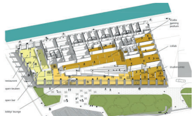
Figure 65: Diagram showing the ground floor, semi-public, functions (KCAP Architects)
