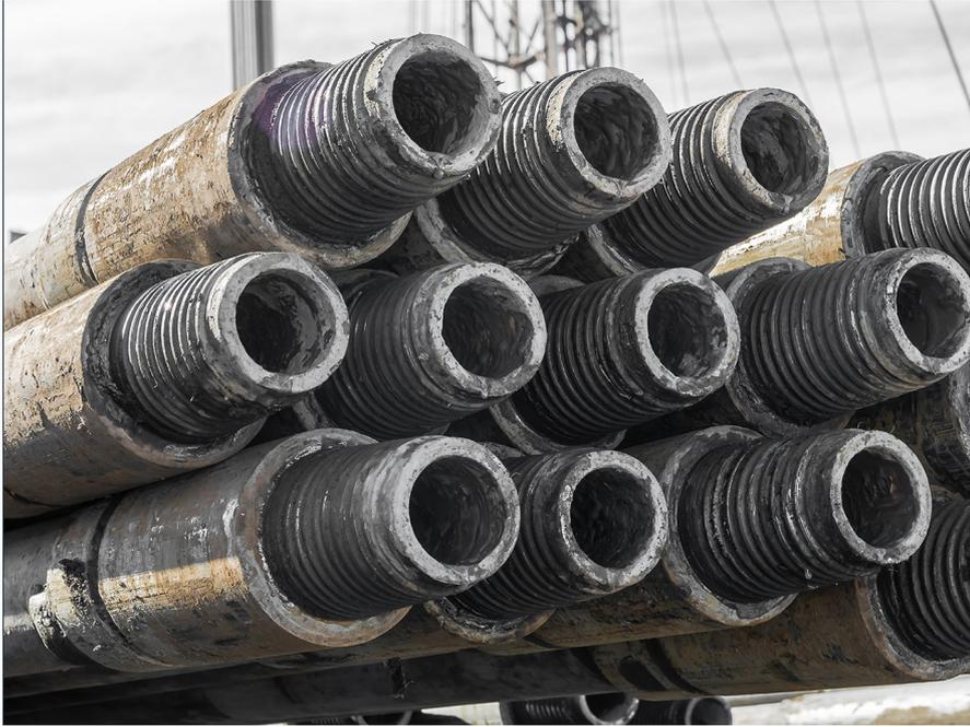
Figure 2.5: Example of drill pipe connectors utilized in the industry [Bormill Inc. \[2019\]](#)
