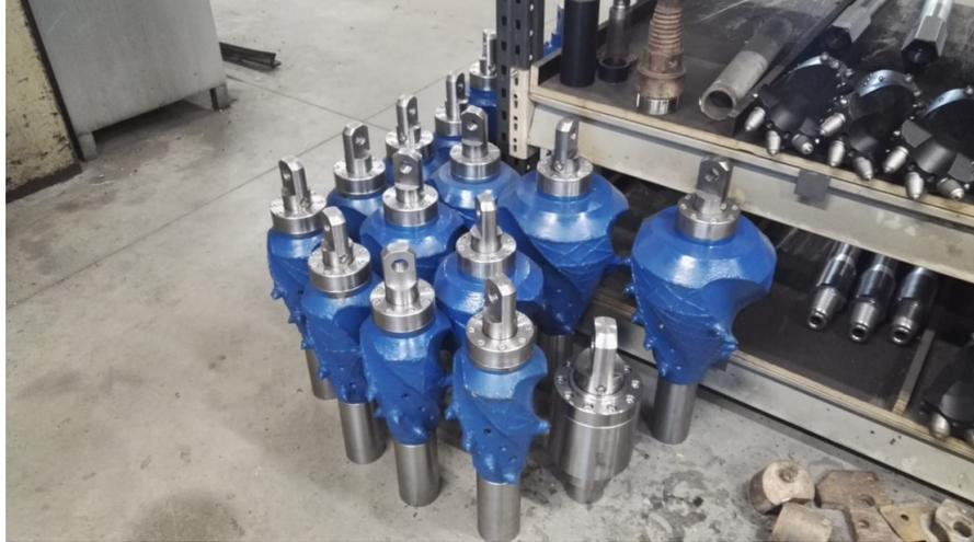
Figure 2.7: Example of rock reaming tools utilized in the industry (Drillingbits.eu [2019])
