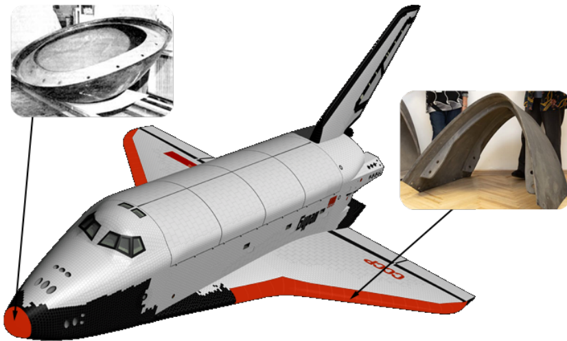
Figure 2.5: C/SiC nose cap and leading edges (highlighted in red) of the Soviet Buran space shuttle [57] [58].
