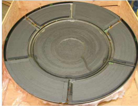
Figure 2.8: Internal view of Lockheed's carbon/carbon hot structure heat shield, displaying its integrated stiffeners [11].
