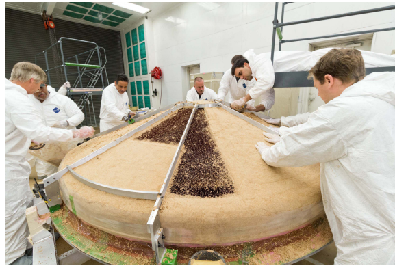
Figure 2.2: Construction of the monolithic SLA-561V heat shield for the Mars InSight lander [32].
